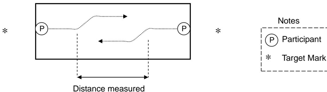
Fig.3 Collision avoidance measurement (ground plan)
