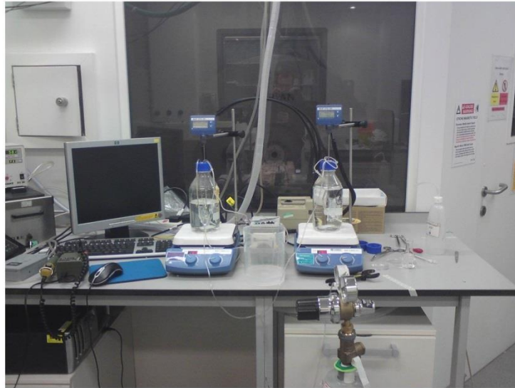
Figure 6.1.1: Potassium Ion Doped and Control aCSF Set-up for Pumping to the Chamber.
