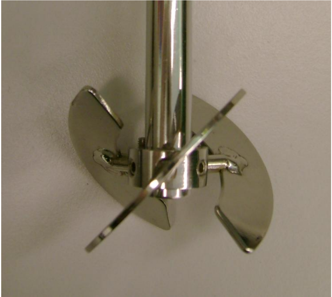
Figure 2.3: Stainless steel three-bladed impeller ( D = 67 mm) with a dimensionless power number of 0.97 (measured at Re = 16,000 ) and a blade angle of 45^\circ .
