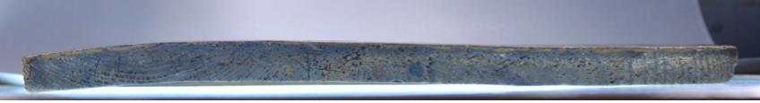
Figure 2: In the Twelve Feasts icon, the wooden panel substrate has bowed towards the painted surface. This shows the warping from the bottom of the icon, with its painted surface facing up. Image courtesy of Bee Keyzer, owner.
