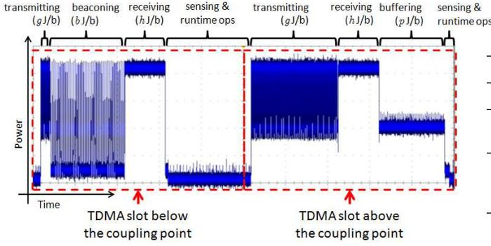
Figure 2. Energy profile of a TelosB sensor node within an undercoupled and an overcoupled TDMA slot during the active period. The indicated metrics (in Joule-per-bit) are defined in Table I.
