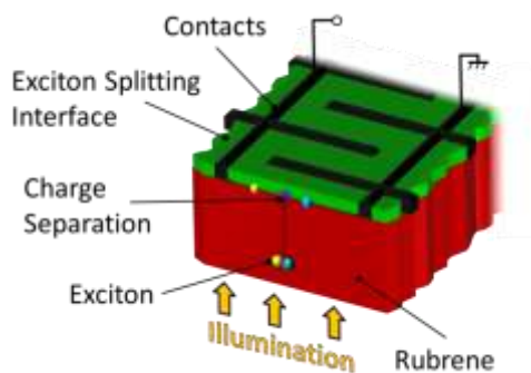
Figure 7-1 Concept of a solar cell device based on a thinly cleaved rubrene sample.
