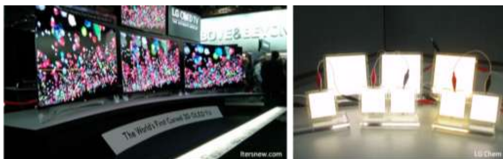
Figure 1-2 Left, Worlds first curved 3D OLED TV produced by LG. Right, OLED white light source panels produced by LG Chem.
