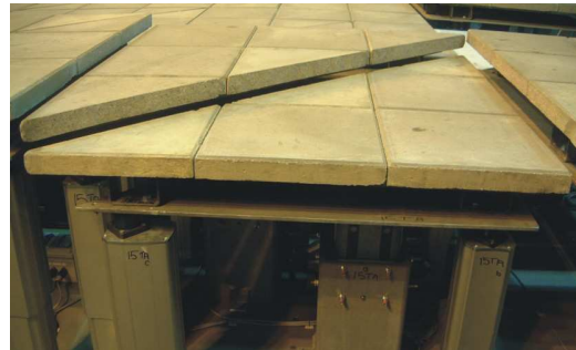
Fig 3. Split-square module : each triangle set to a different height
