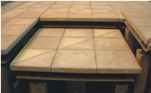
Fig 2. Square module : lowered position
