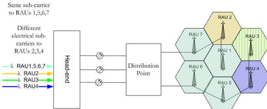
Figure 8: Hybrid simulcasting / 1:1 electrical sub-carrier→RAU mapping scheme
