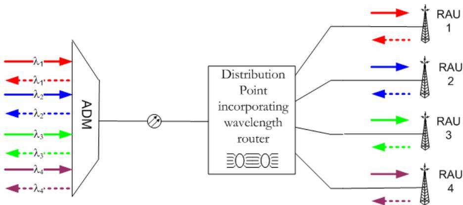
Figure 3: 1:1 Static wavelength mapping scheme
