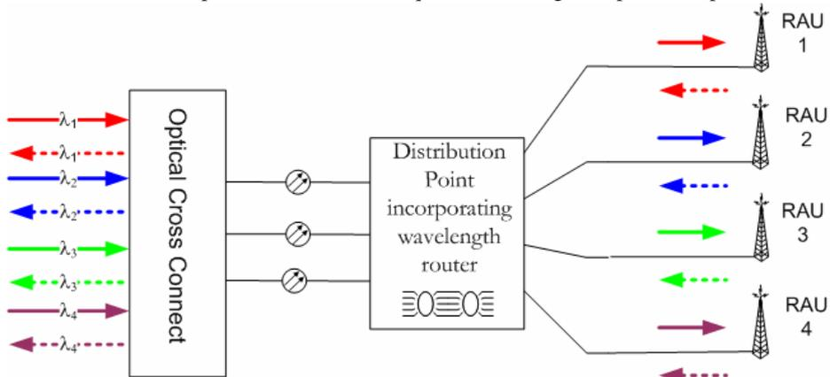
Figure 4: 1:1 Dynamic wavelength mapping scheme
