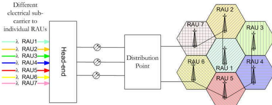
Figure 7: 1:1 electrical sub-carrier→RAU mapping scheme
