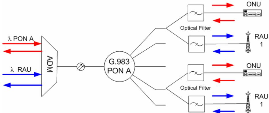
Figure 2: 1:n Static wavelength mapping scheme
