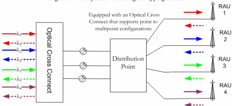
Figure 5: 1:(1 or n) Dynamic wavelength mapping scheme
