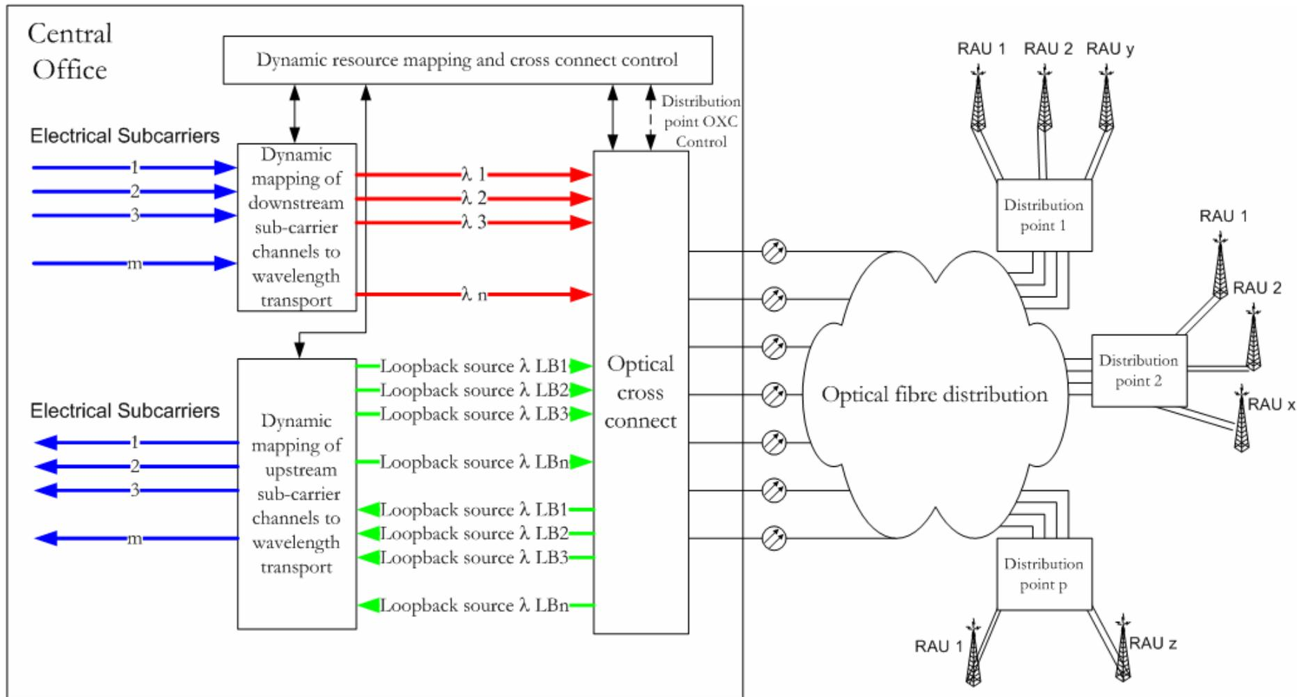
Figure 1: Wireless capacity reconfiguration on a WDM optical network support radio services.
