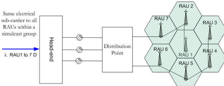
Figure 6: Simulcast electrical sub-carrier mapping scheme
