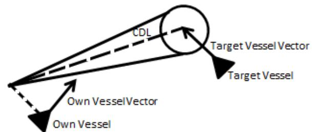
Figure 1. Construction of a collision danger sector (CDS).
