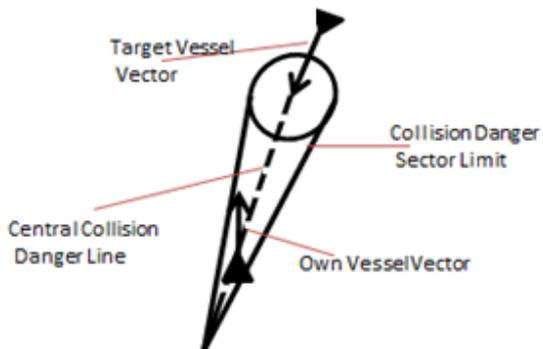
Figure 2. Example of a CDS trial with another vessel approaching at 30 degrees, the tip of the own ship vector is within the CDS indicating a collision risk.
