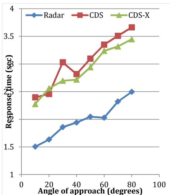
Figure 4. Response time with increasing angle of approach in CDS (Collision Danger Sector), Radar, and variant CDS-X conditions.
