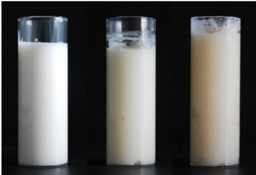
Figure 2. A photograph showing the gas-monomer liquid foam 5 min after mechanical frothing. Left: AESO 1 (0 wt.-% BC), middle: AESO 2 (0.5 wt.-% BC) and right: AESO 3 (1 wt.-% BC).
