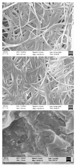
Fig. 2 Scanning electron micrographs showing the morphology of neat and modified BC. Top: Neat BC, middle: C<sub>6</sub>-NDBC and bottom: C<sub>6</sub>-FDBC.
