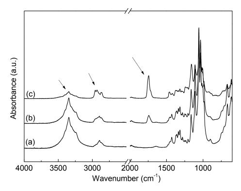
Fig. 1 ATR-IR spectra of neat and hexanoic acid modified BC. (a) Neat BC, (b) C<sub>6</sub>-NDBC and (c) C<sub>6</sub>-FDBC.
