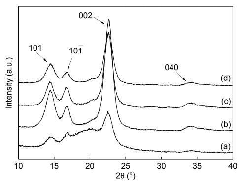
Fig. 3 XRD spectra of hexanoic acid modified BC. (a) C<sub>6</sub>-NDBC, (b) C<sub>6</sub>-FDBC, (c) never-dried BC and (d) freeze-dried BC.
