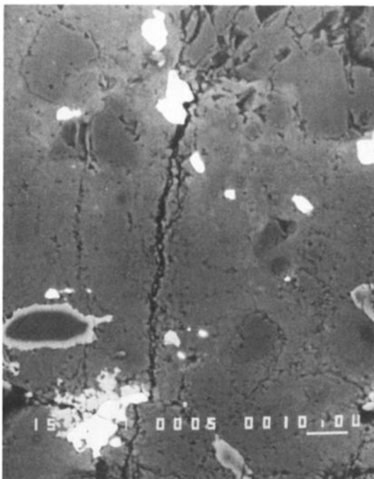
Figure 3. Broken Fe-doped cell after 2 hour experiment. The reacted zone next to the furnace is clear, as well as a darker zone around that where no reaction is apparent in the Fe, but the pressure medium is better sintered than further out. The inset shows a backscattered electron image of the region immediately next to the furnace. The bright regions consist of Fe and 'FeO' in intimate contact, the dark grains are MgO with (Fe,Mg)O solid-solution rims and the intermediate grey groundmass consists of magnesia, alumina and silica with no apparent structure at the resolution of the microprobe.
