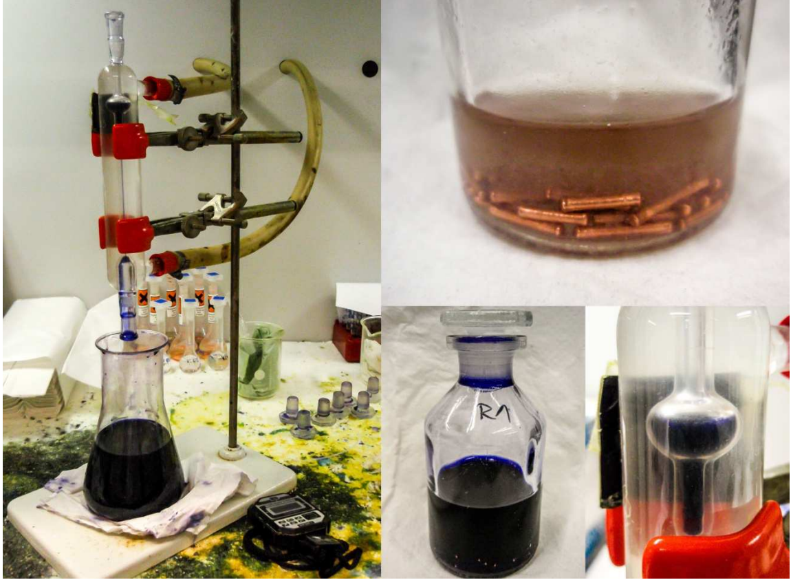
Figure 5.6: Capillary viscometer (left and bottom right), defibred paper sample in water with copper wire, used to mechanically defibre the samples (top right) and a cupriethylenediamine (CED) solution of paper (bottom middle).
