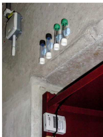
Figure 4.4: HOBO data logger (bottom) and four diffusion tubes in the repository without air filtration (40A), in the general environment. The top left data logger is a part of the regular monitoring, carried out at the Nationaal Archief.
