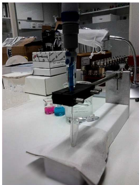
Figure 5.8: pH measurement using the micro electrode.
