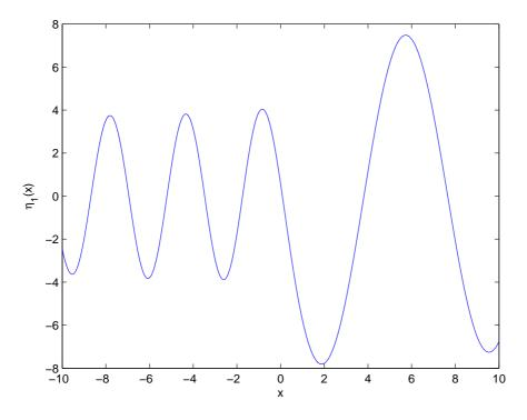
Figure 2.3: Free Surface Profile,  $\eta_1(x), U=0.8>U_{min}=0.67$
