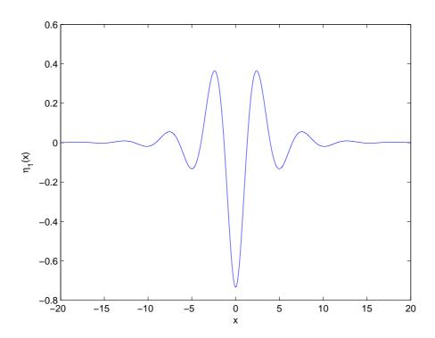
Figure 2.2: Free Surface Profile,  $\eta_1(x), U = 0.6325 < U_{min} = 0.67$
