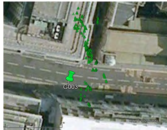
Figure 23. Conventional GNSS positioning solution using weighted least square (WLS) at site G003.
