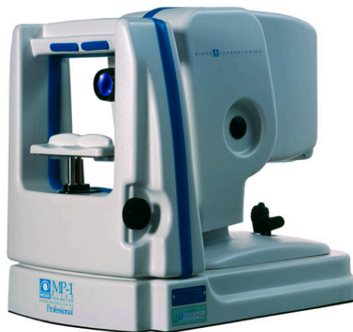
Figure 2.2. The MP-1 from Nidek Technologies (Italy), comprising an infrared fundus camera and an LCD display.
