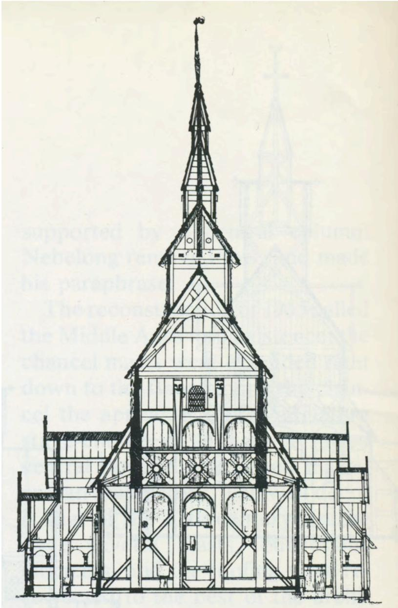
Figure 8: Borgund stave church: plan and long section. (Bugge G. *Stave-churches in Norway*. Dreyers Forlag A/S (1983) p64.)
