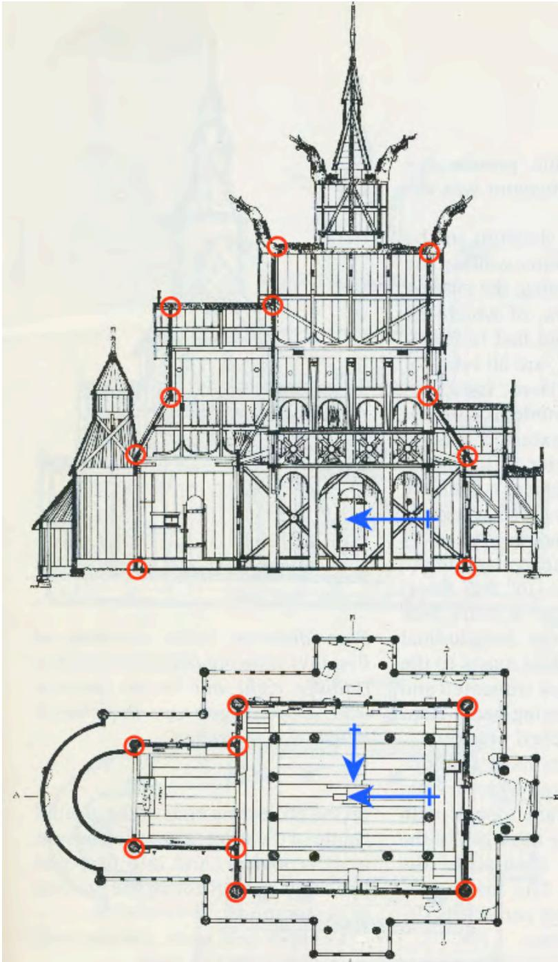
Figure 11: Borgund stave church: plan and long section. (Limits to the medieval core denoted by red circles.)
