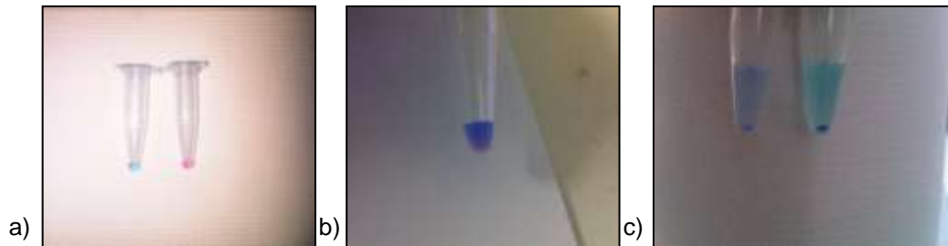
Figure 2.9: a) Differentially labelled sample (blue, left) and control (red, right) DNAs prior to combination. b) Combined labelled and control DNA prior to co-precipitation. c) Precipitated labelled and control DNAs prior to resuspension. A strong purple pellet is seen on the left and a blue pellet on the right indicating poor labelling or precipitation.
