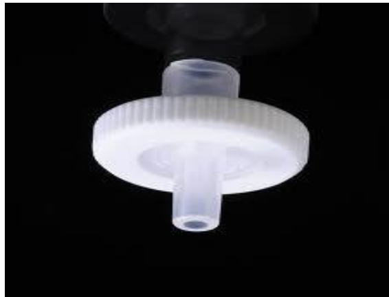
Figure 5.2- The commercial syringe filter unit (13 mm diameter) was used as the basis for the simplified geometry model in Figure 5.3.
