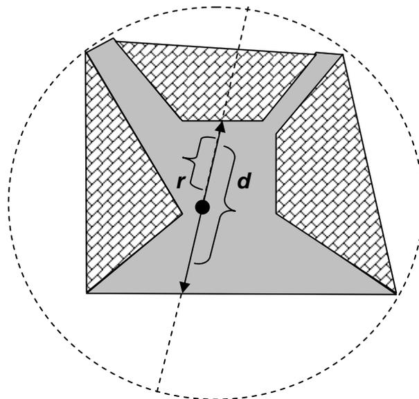
**Figure 1.** Isovist of an observer and the corresponding radial ( $r$ ) and diametric ( $d$ ) lengths.
