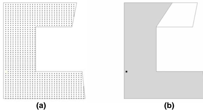
**Figure 2.** (a) A simple indoor open space with a dense mesh of potential observers, and (b) isovist of the observer with the largest isovist area
