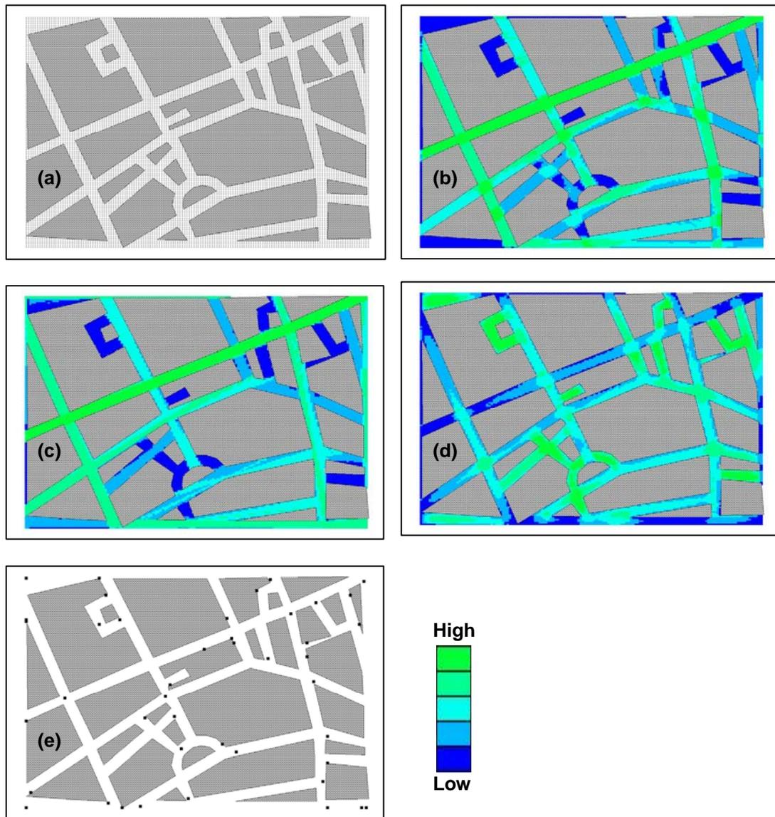
**Figure 6.** (a) Aldwych area in Central London with the dense mesh of observers, and the maps of (b) isovist area, (c) maximum diametric length, (d) circularity, and (e) optimal observers from ROPE algorithm.
