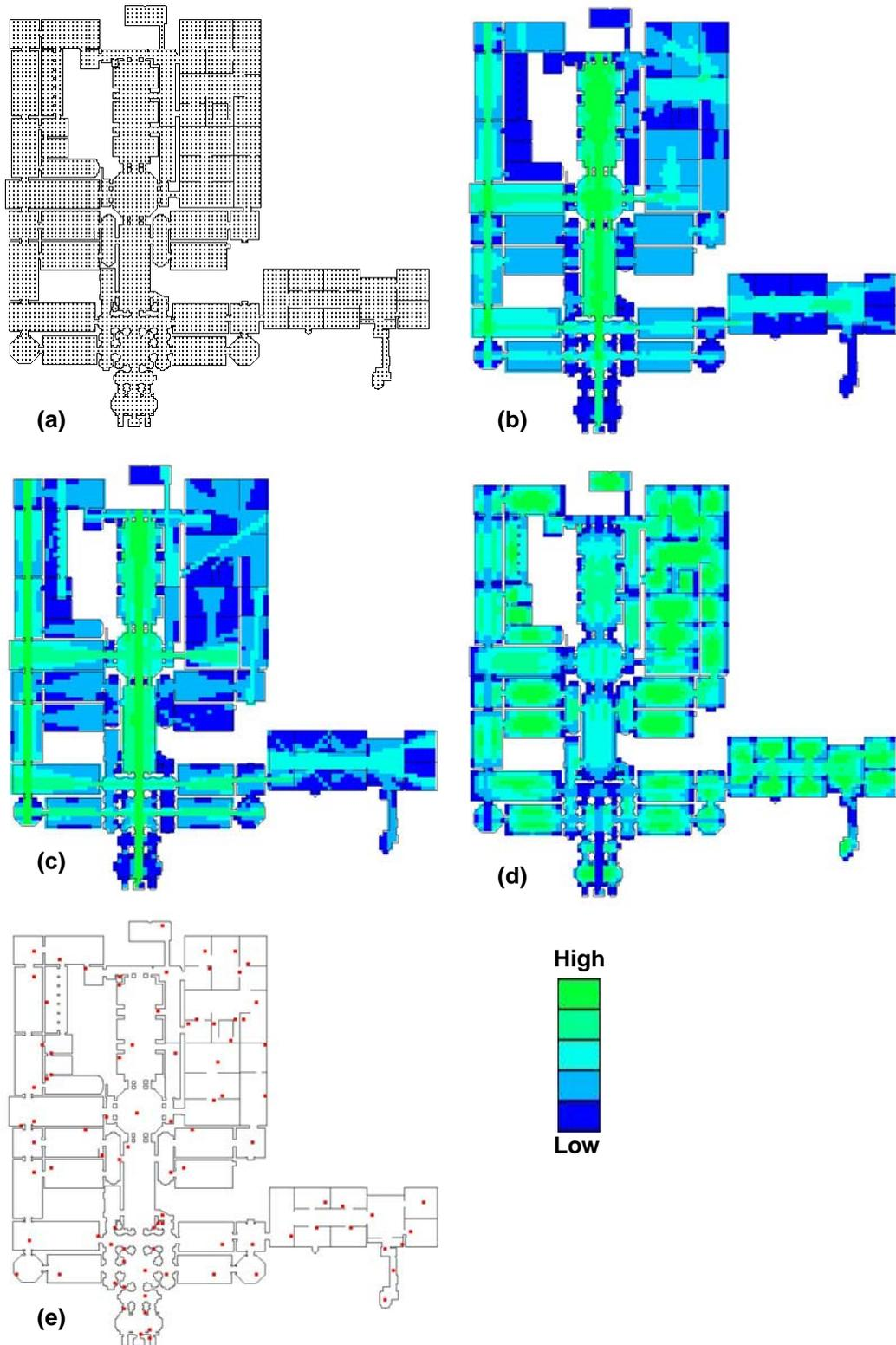
**Figure 5.** (a) Tate Britain Gallery with the dense mesh of observers, and the maps of (b) isovist area, (c) maximum diametric length, (d) circularity, and (e) optimal observers from ROPE algorithm.
