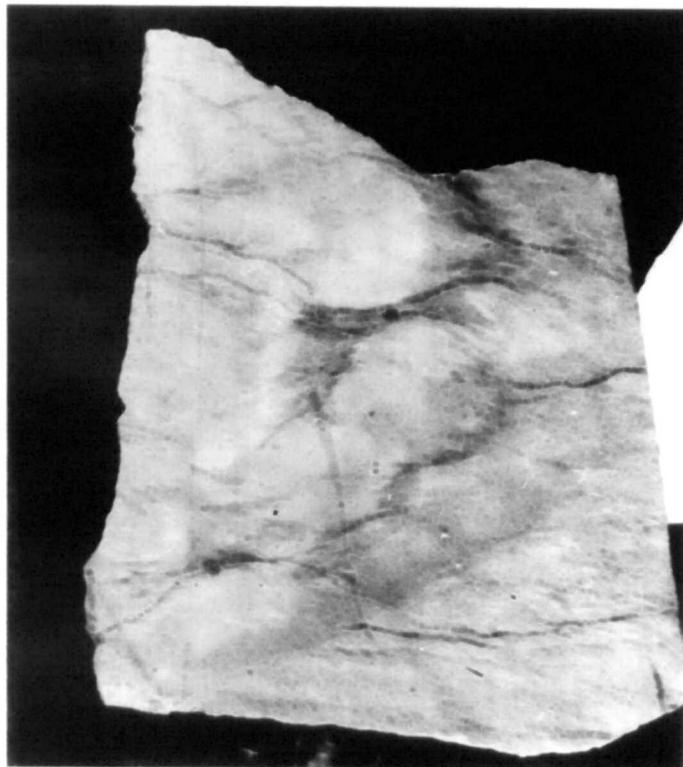
Plate 3.8. Small-scale shearing of a slump resulting in a shredded appearance. Well 2\7-B11, depth 10635', Tor Fm.
