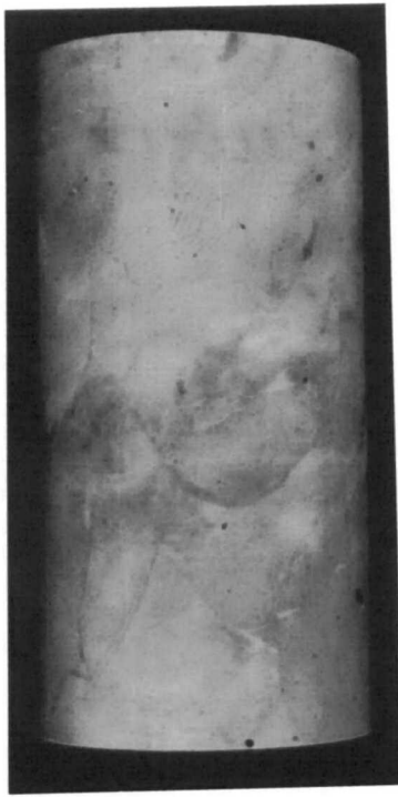
NEOC17: L. Ekofisk Fm., Depth 3156.2m, Lithological variations picked out by syn-sedimentary fractures.
