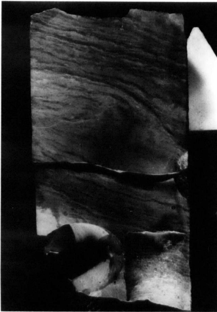
Plate 3.6. A small scale slump further deformed by small scale extension. Well 2\7-A20, depth 9837.5', Ekofisk Fm.
