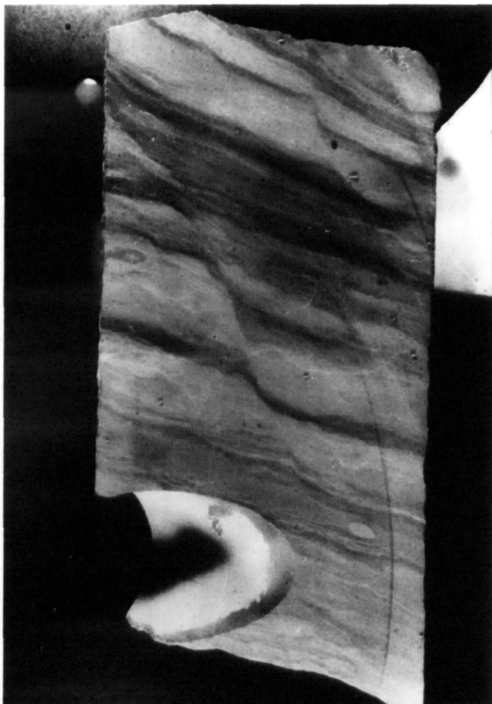
Plate 3.9. Faulting in a chalk which sustained a high fluid content at the time. Well 2\7-B11, depth 10614', Hod Fm.
