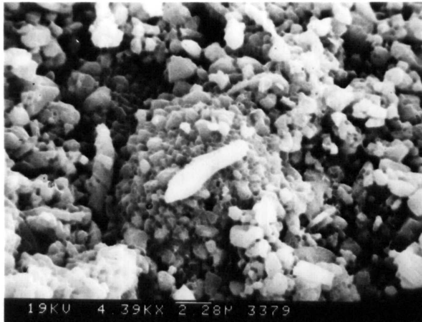
Plate 4.1. Scanning electron micrograph for a sample of Stevn's Klint chalk subject to approximately 28% axial strain.
