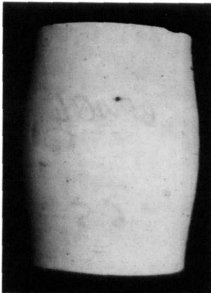
Plate 6.5. Sample BHWC4, isotropically consolidated to 40MPa. Undrained shear has resulted in a barrel shaped sample.
