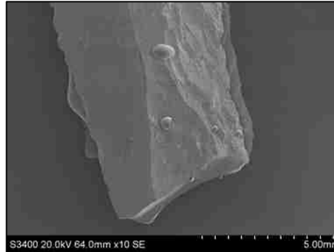
Figure D.12. SEM image of snapped microdrill replica in unit 13465, Building 60
