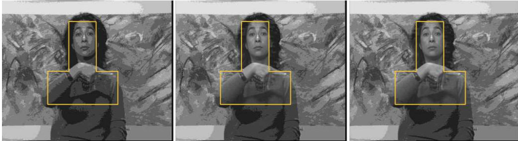
Figure 3.13: ROI-based incremental transform decomposition. An example frame with terminating bitplanes 5, 2, 0 is shown (from left to right).
