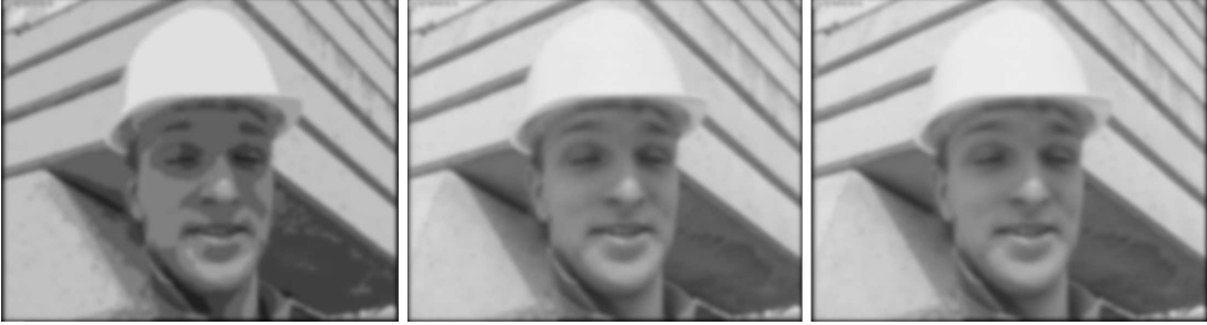
Figure 3.9: Representative output frame for terminating the computation at n = \{5, 2, 0\} bitplanes (shown from left to right) for the 12 \times 12 Gaussian filtering.
