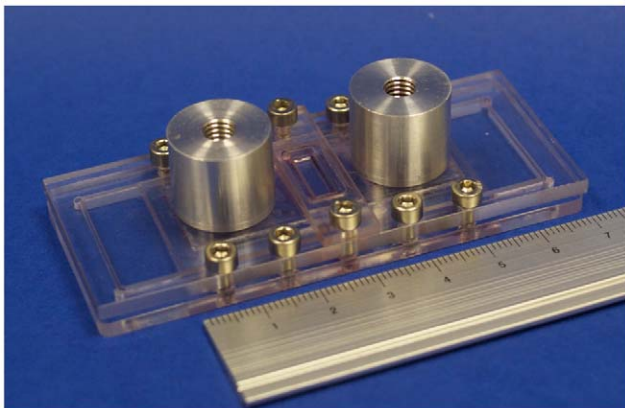
Figure 2. Photograph of the assembled modular culture device with the re-sealable lid attached. doi:10.1371/journal.pone.0052246.g002
