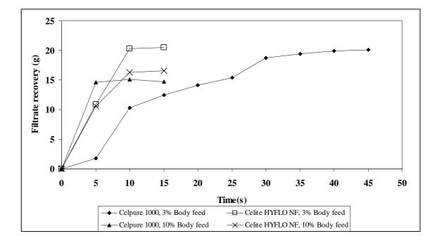
**Figure 5.10**Fraction IV paste filtrate recovery over time(s). 20g of FIV paste was filtered through a K900 Seitz filter using a Sartorius SM16249 filter housing. The filtration process was stopped when the filtrate started to foam.
