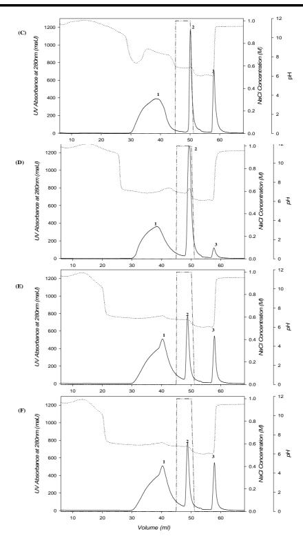
**Figure 5.4**Elution profiles of Fraction IV filtrate on 1mL pre-packed columns: (C) & (E) Fractogel EMD TMAE column, and (D) & (F) Hitrap Q Sepharose FF. Peak 1 represents the wash of unbound protein with 20mM Phosphate at pH 7 in profiles(C) & (D); 20mM Phosphate, 30mM NaCl at pH 7 in profiles (E) & (F). Peak 2 shows a salt step elution to 1 M NaCl, Peak 3 is a 0.5M NaOH wash. Symbols are: (—) Absorbance, (---) NaCl concentration, (---) pH.
