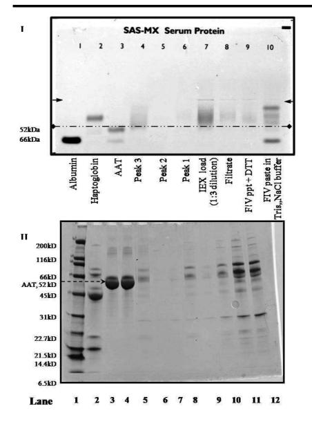
**Figure 5.2**Initial process trial, based on Kee*et al.* conditions: Analysis of process samples for the presence of AAT from successive steps in the purification of AAT from Cohn FIV precipitate by I) electrophoresis on a 1% agarose gel. II) SDS-gel electrophoresis. Samples (4-20% Pierce gel, Coomassie blue stain).
