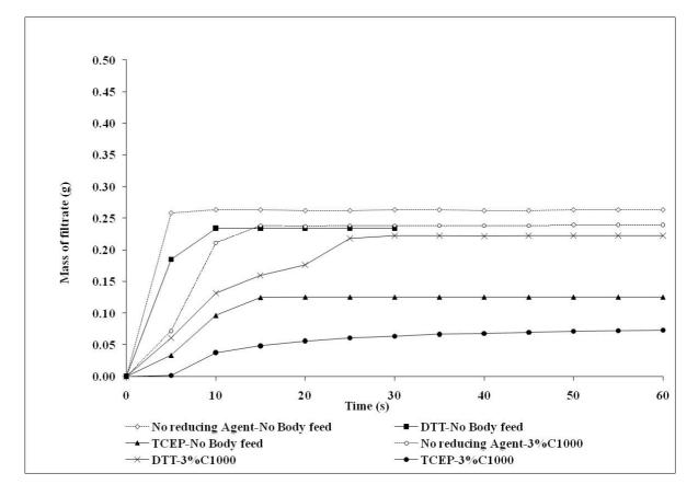
**Figure 5.11**Filtration curves for the recovery of Fraction IV filtrate over time(s). 20g of FIV paste was filtered through a K900 Seitz filter using a Sartorius SM16249 filter housing.
