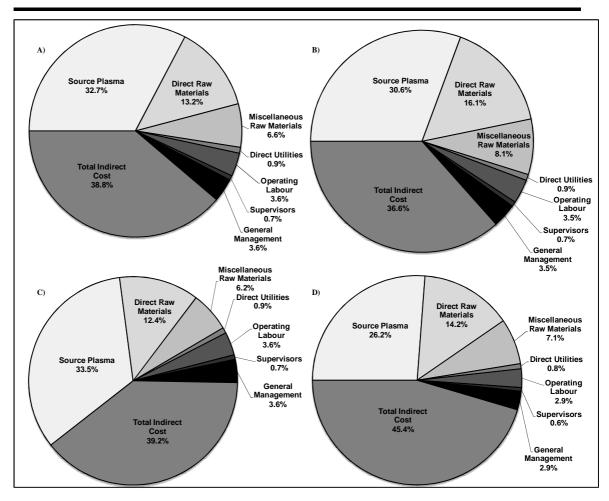
**Figure 4.3**Process change scenario cost comparisons of (A) the base case, (B) a 'forced' minor change -an addition of a virus inactivation step, (C) a 'forced' major change where the formulation is modified (D) a major change- where B+1 precipitation is replaced with a chromatography-based purification step.
