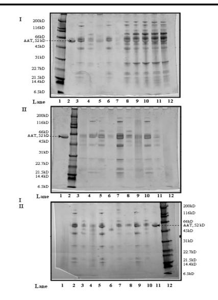
**Figure 5.6** Analysis of samples from successive steps in the purification of AAT from Fraction IV precipitate, and preparative anion exchange runs using SDS-gel electrophoresis. Samples were applied to a 4-20% Pierce gel and electrophoresed at 120V for 45 minutes. The gel was stained with Coomassie blue.
