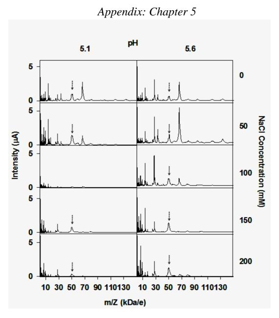
**Appendix 5 - Figure 1**SELDI-TOF-MS spectra representing protein profiles portraying the impact of further buffer conditions on the binding intensity and isolation of AAT using the 'Q10' ProteinChip. The buffer conditions shown are a combination of pH 5.1-5.6 and 0-200mM NaCl.
