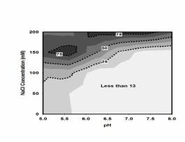
**Figure 6.7** The percentage purity of AAT (AAT/ Total Protein) when fractionated using the SELDI-TOF-MS 'Q10' ProteinChip under a range of pHs and NaCl concentrations.
