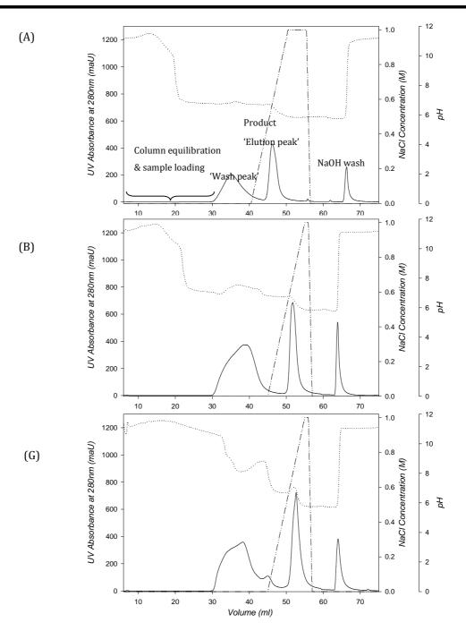
**Figure 5.3**Elution profiles of Fraction IV filtrate on 1mL pre-packed columns: (A) & (B) Fractogel EMD TMAE column, and (G) Hitrap Q Sepharose FF. Peak 1 represents the wash of unbound protein with 20mM Phosphate at pH 7, Peak 2 shows a 10 column volume salt gradient elution (0-1 M NaCl), Peak 3 is a 0.5M NaOH wash. (A) represents a load of 4.5mL and (B)/(G) a 9mL load. Symbols are: (—) Absorbance, (---) NaCl concentration, (---) pH.
