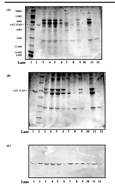
**Figure 5.13** Analysis of samples from successive steps in the purification of AAT from Fraction IV precipitate using SDS-gel electrophoresis and Western blot analysis. Samples were applied to a 4-20% Pierce gel and electrophoresed at 120V for 45 minutes. For SDS PAGE analysis the gels were stained with Coomassie blue.
