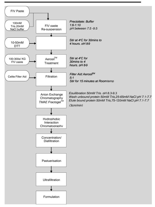
Figure 5.1Kee*et al.* Method for the purification of AAT from Human Plasma FIV precipitate.
