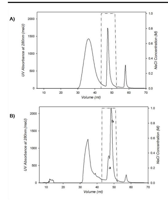
**Figure 5.12**Elution profiles of Fraction IV filtrate on 1mL pre-packed columns: (A) Fractogel EMD TMAE column, and (B) Hitrap Q Sepharose FF. Columns are equilibrated to pH 7 with 20mM Phosphate buffer, protein is loaded at pH 6.2, Peak 1 represents the wash of unbound protein with 20mM Phosphate at pH 7, Peak 2 (a-b) shows a step elution to 1 M NaCl, Peak 3 is a 0.5M NaOH wash. Symbols are: (—) Absorbance, (- -) NaCl concentration
