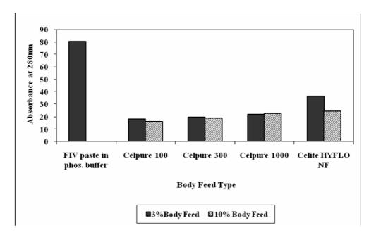
**Figure 5.8**The impact of filter aid body feed type and percentage body feed on protein concentration. 20g of FIV paste was filtered through a K900 Seitz filter using aSartorius
