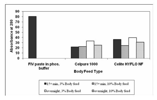
**Figure 5.9**The impact of filter aid body feed type, percent body feed, and mixing time on protein concentration. 20g of FIV paste was filtered through a K900 Seitz filter using a Sartorius SM16249 filter housing. The filtration process was stopped when the filtrate started to foam.
