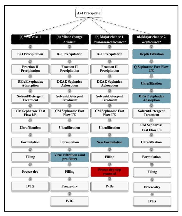
**Figure 4.2.** Process change scenariosinvestigated: (a) the base case (b) a minor change with the an additional virus inactivation step, (c) a major change where the formulation process is modified and the freeze dryer step is removed, and (d) a major change where Fraction B+1 precipitation is replaced with a chromatography-based purification
