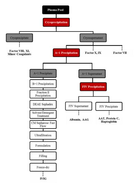
**Figure 4.1** A process flow sheet depicting and example of a plasma fractionation scheme based on a combination of Cohn (Method 6) and Kitsler and Nitchmanmethods, with a focus on the IVIG production stream.
