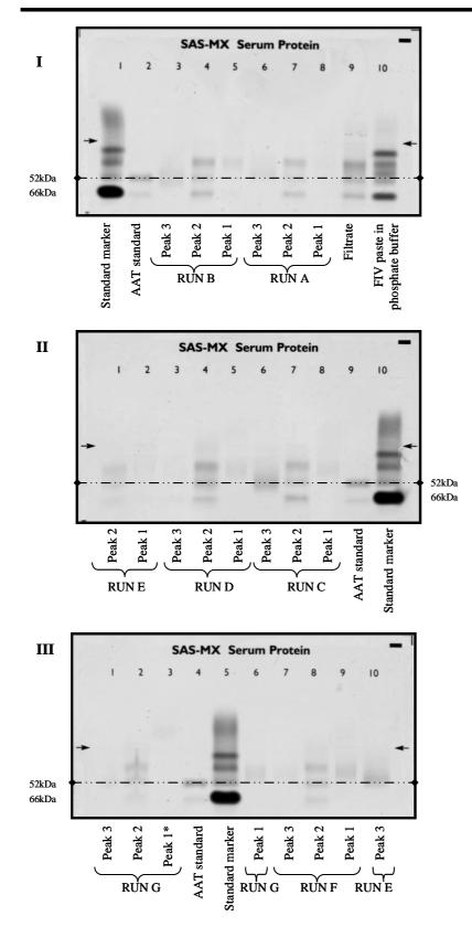
**Figure 5.5**Analysis of process samples for the presence of AAT by electrophoresis on a 1% Agarose gel. Standard marker used is N/T protein Control LC® (Dade-Behring). Samples were electrophoresed at 80V for 30 minutes.
