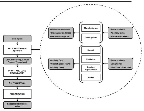
**Figure 3.6**A Simplified schematic of the main inputs and outputs of the proposed framework.
