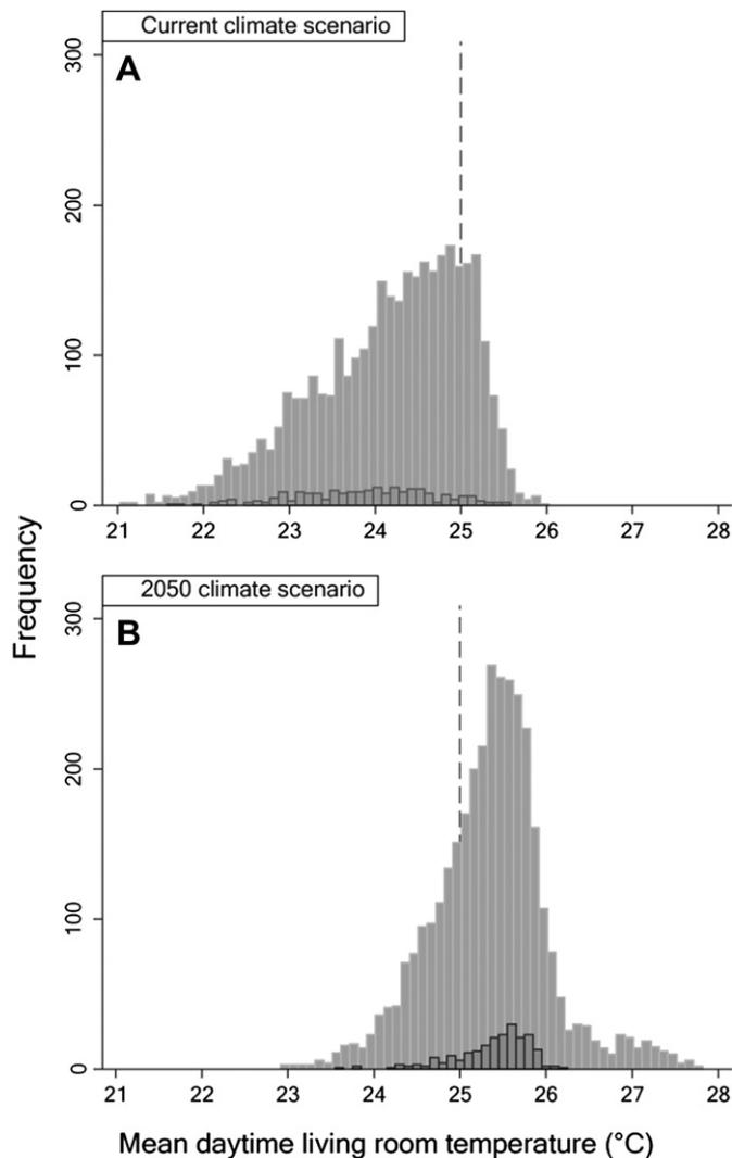
**Fig. 8.** Distribution of simulation results for mean summer (June, July, August) daytime living room temperatures: [A] current climate (CIBSE DSY); [B] future climate (UKCP09 50th percentile of external temperature, 2050s, medium emissions scenario, PROMETHEUS DSY). Dark grey bars in [A] indicate dwellings with no retrofitting; dark grey bars in [B] indicate dwellings with full retrofitting.
