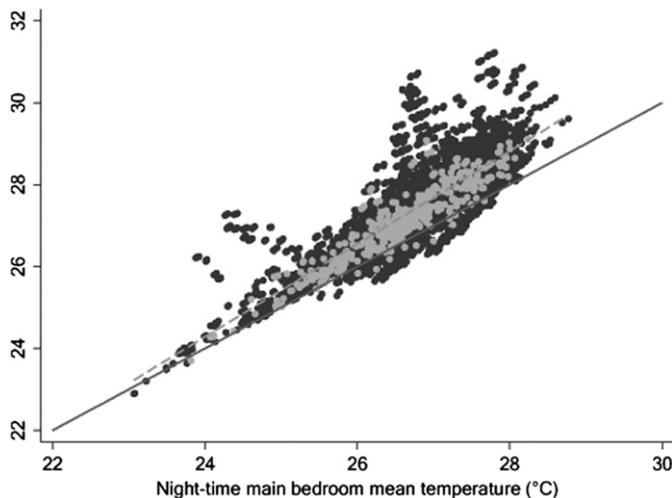
**Fig. 7.** Relationship between mean daytime living room temperature and mean night time main bedroom temperature. Light grey dots indicate dwellings with full retrofitting of energy efficiency measures; solid line is the line of equality; dashed line shows the fitted values of the regression of daytime living room mean temperature on night time bedroom mean temperature.
