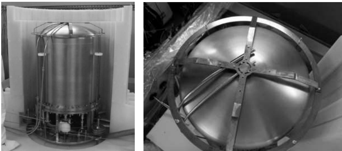
Figure 3. Left: ZEPLIN-III partially surrounded by the polypropylene slabs of the veto system. Two pipes of the source delivery system are attached to the vacuum dome. The detector leveling system with pulley wheels and cables can be seen at the bottom of the detector. Right: ZEPLIN-III viewed from the top. The gamma source was delivered through the pipe above the center of the detector, while the neutron source was placed on the top 5 centimeters off-centre.
