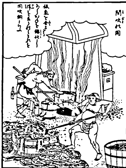
Fig. 6. Removing the copper in disc-shaped layers from the melting furnace. Japan.
