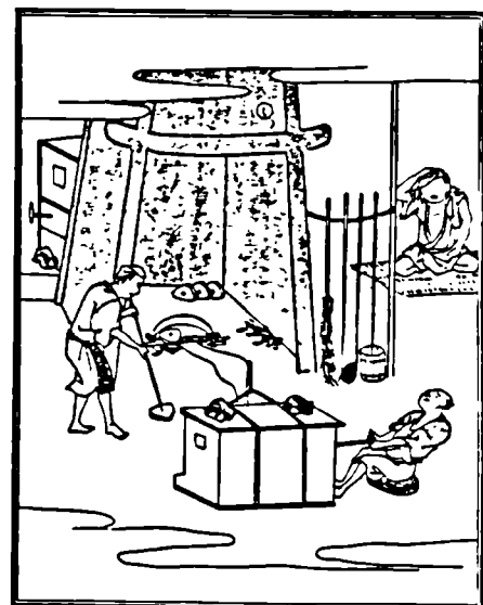
Fig. 7. Converting copper sulphide (regulus) into metallic copper by a blast of air. Japan.
