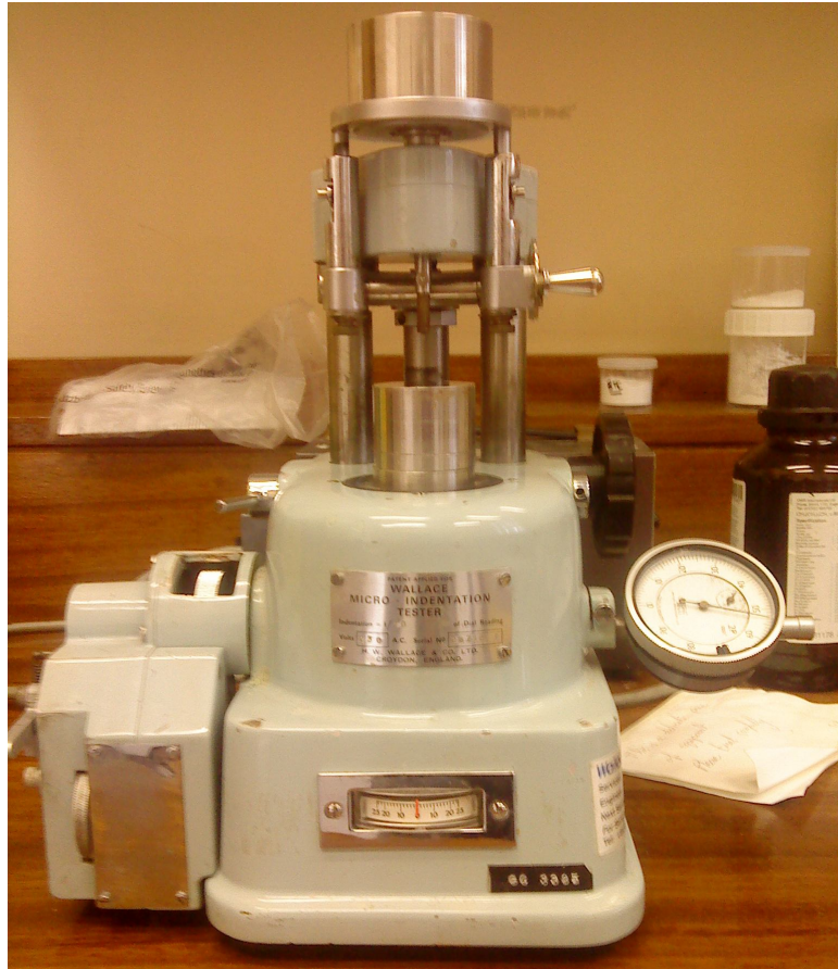
Figure E-1: The Vickers micro-indenter employed to determine the effects of acid erosion on human and bovine enamel.
