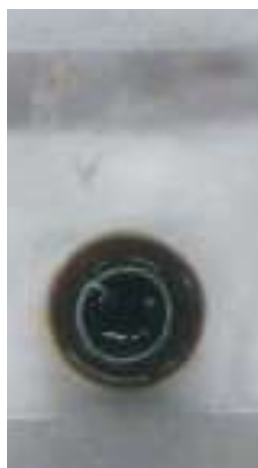
Figure 60 High contrast phantom filled with GNP solutions 4 mgAu/ml (central) and 0.2 mgAu/ml (outer ring)
