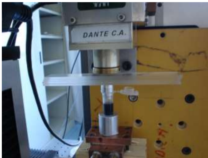
Figure 22 Depth measurement of 8 mgAu/ml GNP sample; a range of Perspex thicknesses were added above the sample to test the effect of depth of measurement on the L-XRF method.
