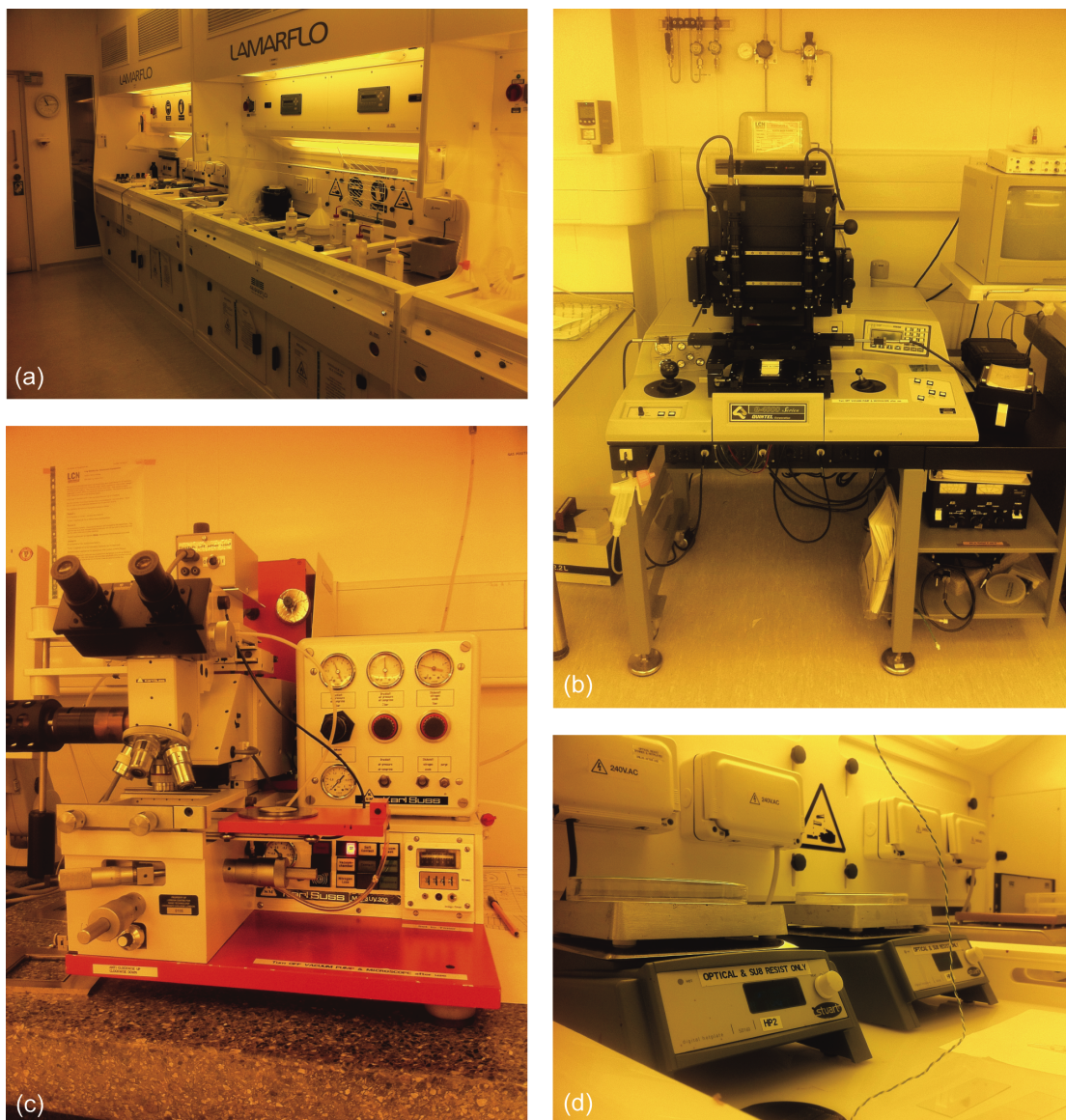
Figure 4.14: a) Wet bench fume cupboards in LCN Class 1000 cleanroom. b) Quintel Q4000-6 Mask Aligner (Class 100 hood). c) Karl Suss MJB3 Mask Aligner (Class 100 hood). d) Hotplates.
