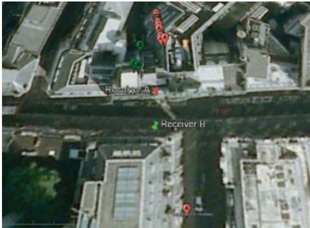
▲ FIGURE 7 True position of receivers against conventional standard point positioning (SPP) solution. Pins show the true positions and bubbles the SPP solutions; the numbers and colors indicate the receiver.
