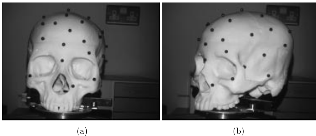
Figure 5.1: Video images of the skull phantom used for the multiple view experiments.
