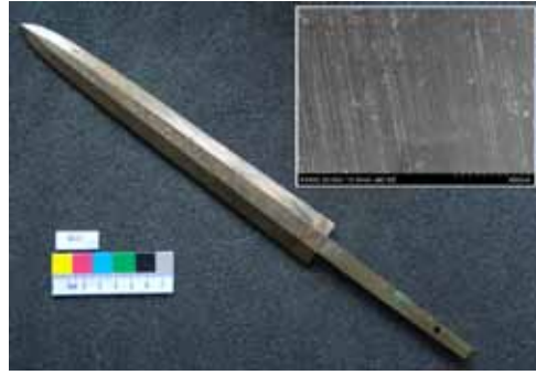
Fig. 12: A bronze lance from the Terracotta Army, with (inset) SEM image of a silicon rubber impression taken on a lance blade, showing the fine polishing marks; their density and parallel arrangement denote the use of a rotary mechanical device.
