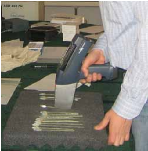
Fig. 9: Analysis of bronze weapons using a portable XRF.
