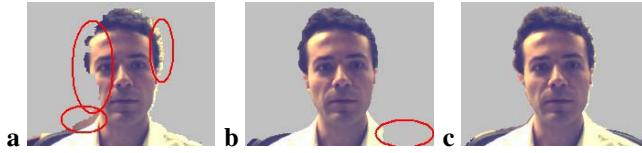
Figure 2: Segmentation by fusing colour, contrast and stereo. Results of three different segmentation algorithms run on the left input image of fig. 1 (see [2] or video in the CD-ROM proceedings for more examples). (a) Stereo-based segmentation. (b) Colour/contrast-based segmentation. (c) The algorithm proposed here, by fusing colour, contrast and stereo achieves more accurate segmentation. The foreground artefacts visible in (a) and (b) (marked in red) are corrected in (c), where the person and chair are correctly extracted. Note, we do not just combine images (a) and (b) to produce (c); see text for algorithmic details.
