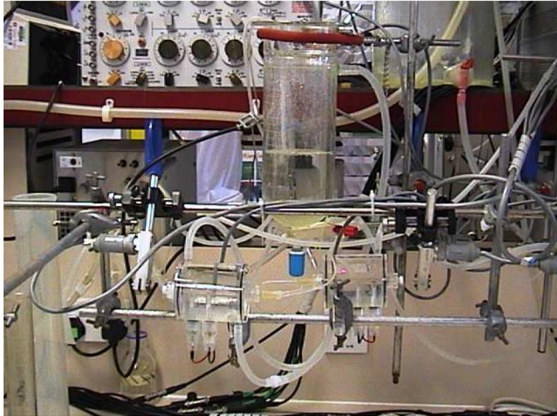
**Figure 17:** Overview of the laboratory set up showing superfusion chambers, organ bath and tubing.
