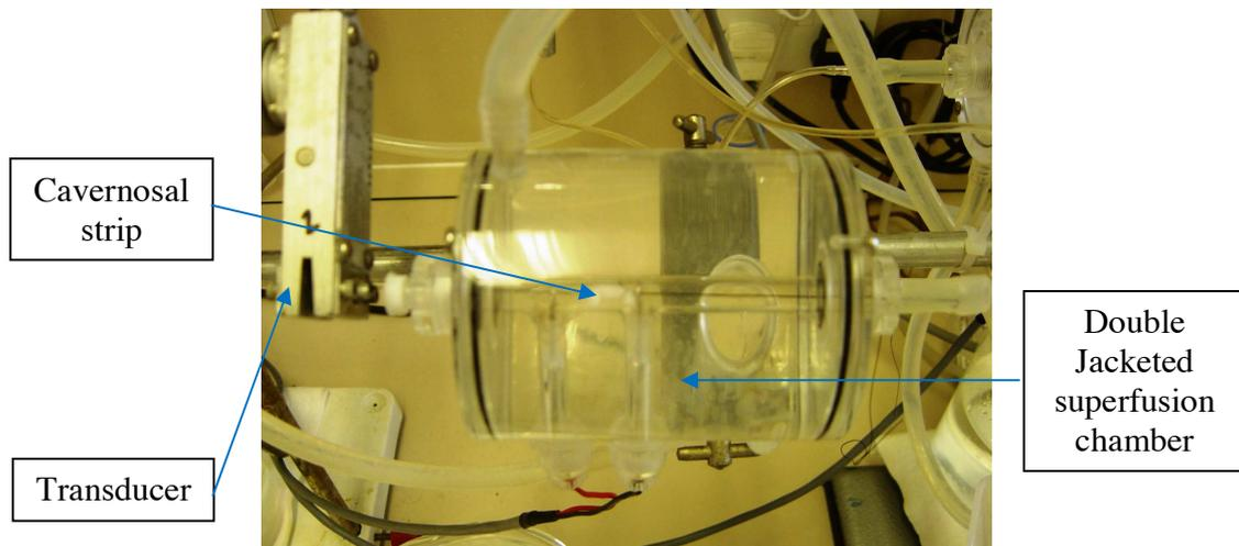
**Figure 16:** Each dissected strip of corpus cavernosum is mounted into a superfusion chamber. One end is attached to a transducer to detect changes in tension and the other end fixed.
