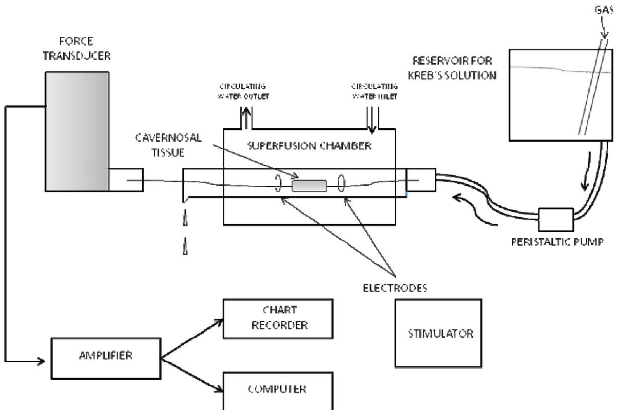
**Figure 18:** Schematic illustration of the experimental set up
