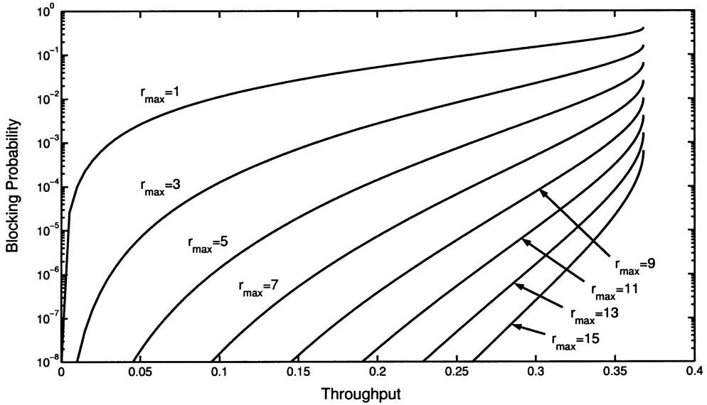
Fig. 4. Blocking probability  $P_B$  versus throughput  $S$ , slotted ALOHA.
