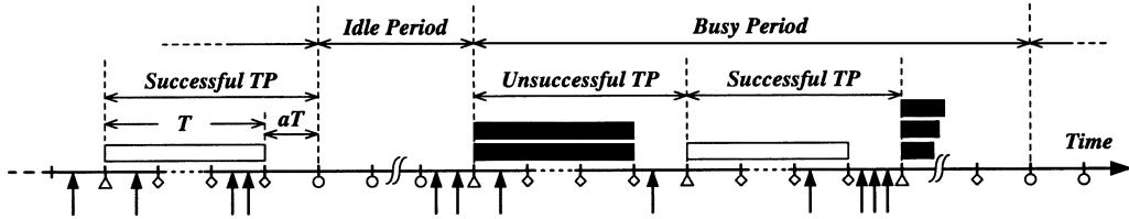
Fig. 12. Busy and idle periods in slotted nonpersistent CSMA protocol. Up arrows point at packet arrival instants. TP is the abbreviation for *transmission period*.
