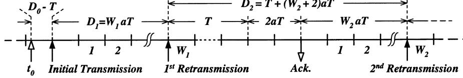
Fig. 2. Access mechanism of slotted nonpersistent CSMA.
