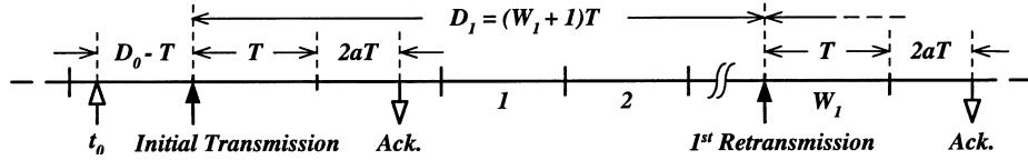
Fig. 1. Access mechanism of slotted ALOHA.
