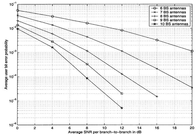
Fig. 12. Average error probabilities for a three-user MTxSINR system with two antennas/MS,  $(K_1, K_2, K_3) = (2, 2, 2)$ , and various number of BS antennas.
