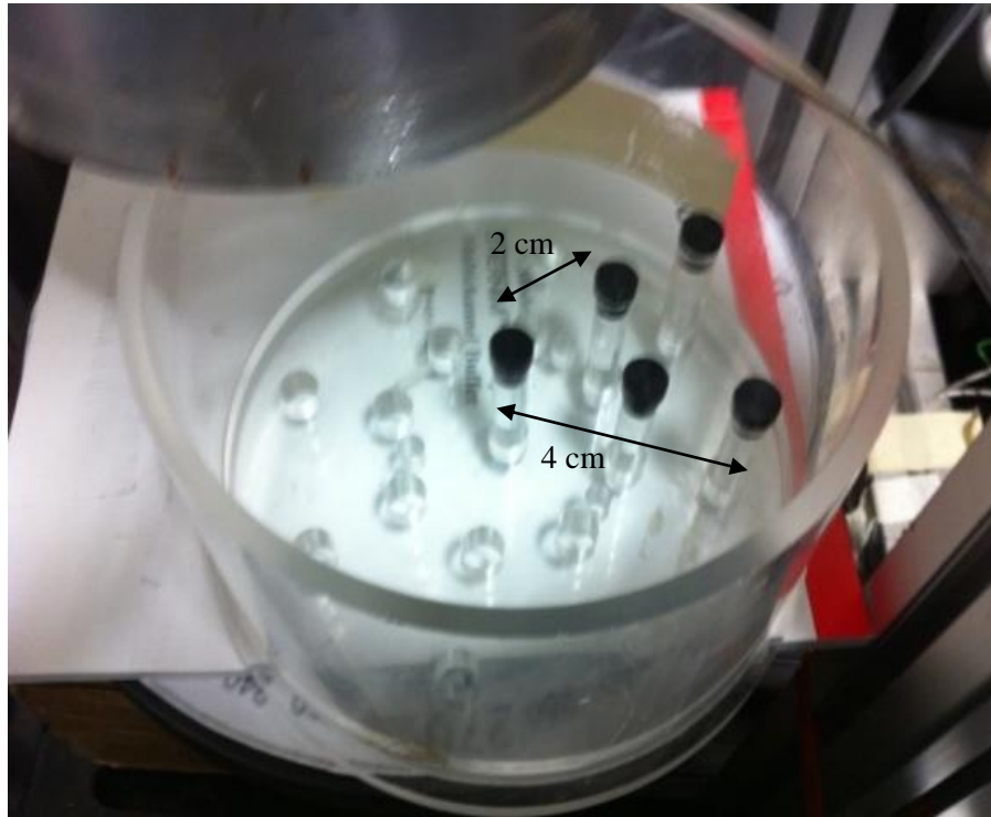
Figure 21: Photographs of the triangles phantom design
