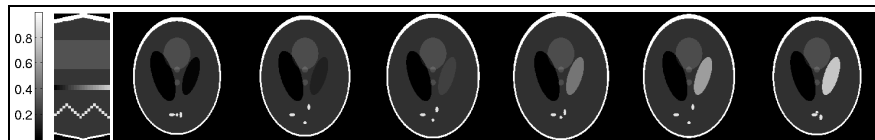
Fig.1: Global (respiratory) motion is simulated by slightly and slowly changing size of the main ellipse. Local motion is simulated by three small ellipses at the bottom. Intensity change from 0 to 1 is visible on the right side ellipse. (Left) y - t profile of the generated sequence. (Right) Extracted frames from the whole sequence at time \{1, 4, 7, 12, 16, 20\} .
