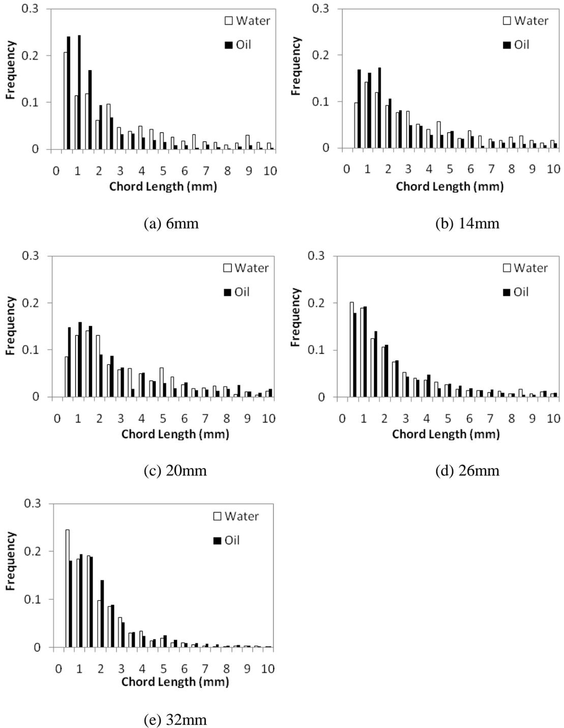
**Figure 4.13:** Chord length distribution of oil drops in water (60% water fraction) at a mixture velocity of 3m/s at (a) 6mm (b) 14mm (c) 20mm (d) 26mm (e) 32mm from the top wall of the pipe. The distributions of the two inversion routes are given – starting from a O/W dispersion (□) and from a W/O dispersion (■).
