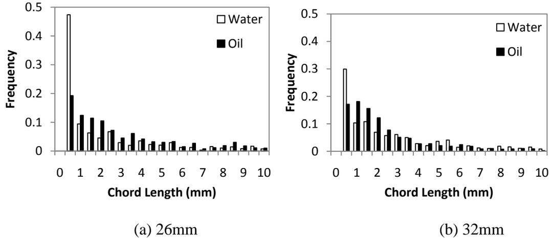
**Figure A-3:** Chord length distribution of oil drops in water (40% water fraction) at various locations from the top wall of the pipe with a mixture velocity of 3m/s. The distributions of the two inversion routes are given – starting from a O/W dispersion ( $\square$ ) and from a W/O dispersion ( $\blacksquare$ ).
