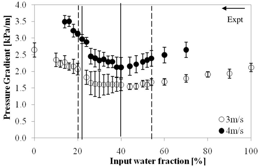
**Figure 4.11:** Comparison of pressure gradient measurement between mixture velocity of 3m/s and 4m/s in an acrylic pipe. The error bars represent the standard deviation of the fluctuations at each phase fraction. The arrow denotes the direction of experiment from water continuous dispersion to oil continuous dispersion. The vertical lines limit the boundaries for phase inversion transition - dotted lines for 3m/s and solid lines for 4m/s.
