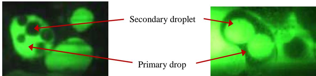
**Figure 2.12:** Visual observations of (a) O/W/O and (b) W/O/W dispersions using LIF technique. The oil phase is shown in black while the water phase is shown in luminous green (Liu et al., 2005).
