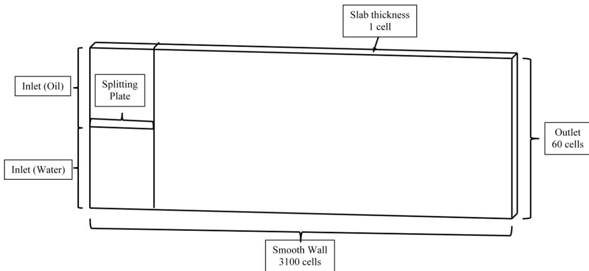
**Figure C-1:** Sample schematics of simulation domain with a vertical height consisting of 60 cells.
