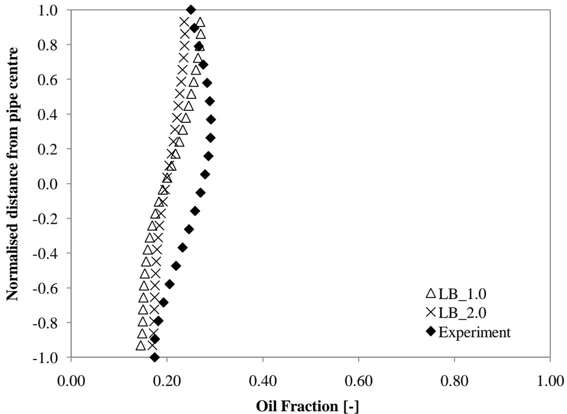
**Figure 8.9:** Effect of turbulent dispersion force coefficient on phase distribution at a mixture velocity of 3m/s and input water fraction of 80%. LB represents the coefficient for the Lopez de Bertodano model in Equation 2.39.
