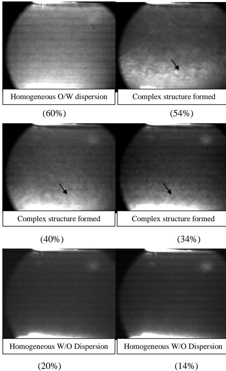
**Figure 4.2:** Visual images are taken in an acrylic pipe using an high speed camera (Model: Kodak HS 4540) at 7m away from the inlet. Mixture velocity is kept constant at 3m/s. The percentage in the bracket represents the input water fraction at which the image is taken. The arrows present samples of complex structures observed in images.
