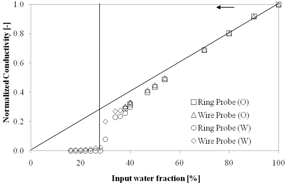
**Figure 4.16:** Normalized conductivity data for an oil/pure water mixture at a mixture velocity of 3m/s using the ring probe and wire probe. The letter in bracket represents initial dispersed phase – (W) water (O) oil. The arrow denotes the direction of experiment and the vertical line denotes the first input water fraction where phase inversion occurs.
