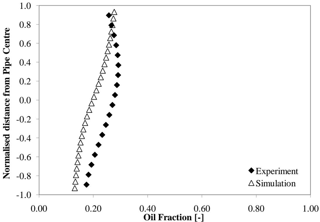
**Figure 8.4:** Comparison between simulated (base) and experimental (ERT) dispersed phase fractions at an input water fraction of 80% and mixture velocity of 3m/s. The simulated data is extracted at 3m from the inlet and the experimental data at 7m where the flow is fully developed.
