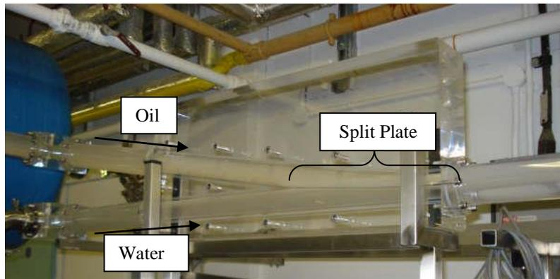
**Figure 3.4:** Acrylic Y-inlet with a split plate to enhance stratification of the oil and water.
