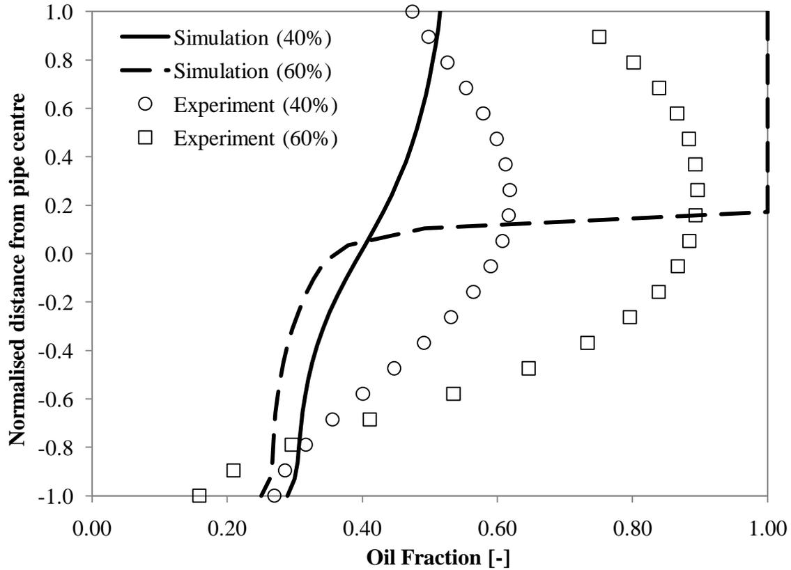
**Figure 8.10:** Comparison between experimental and simulated phase fraction distributions for 40% and 60% input water fractions at a mixture velocity of 3m/s and drop size of 1mm. Oil is set to be the dispersed phase in the simulation. The lift force coefficient is 0.5 and the turbulent dispersion force coefficient is 2.
