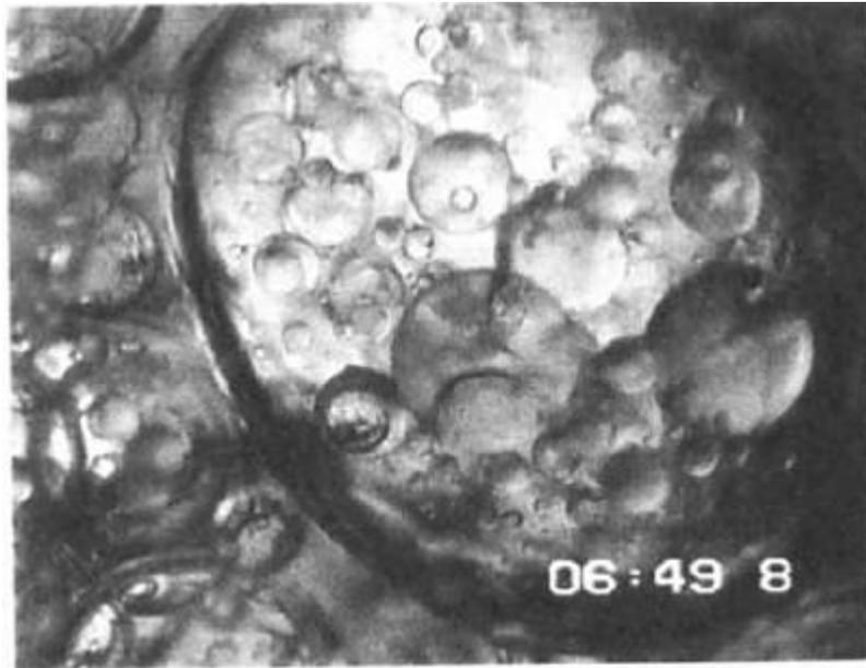
**Figure 2.8:** Droplet in drop for a glycerol/water and chlorobenzene system captured by Sony video printer (Pacek et al., 1994).
