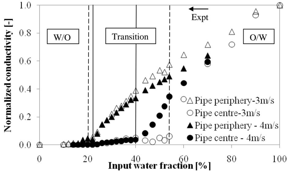
**Figure 4.8:** Comparison of normalized conductivity data for the oil/water mixture at a mixture velocity of 3m/s and 4m/s using the ring probe and wire probe. The vertical lines determine the phase inversion transition at which the first and last near zero conductivity value are recorded using the various probes – dotted lines for 3m/s and solid lines for 4m/s.
