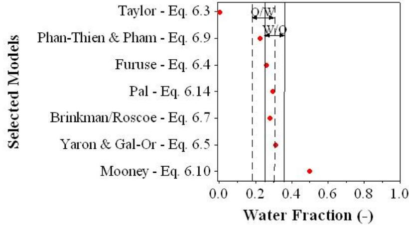
**Figure 6.3:** Predicted inversion points using different dispersion viscosity models against the experimental phase inversion ranges in stainless steel pipe obtained starting from oil continuous and from water continuous dispersions for a water-Marcol 52 mixture. Points in graph refer to the model predictions while the lines represent the experimental phase inversion region.
