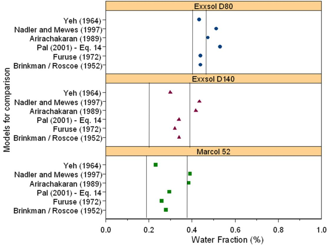
**Figure 6.6:** Comparison between proposed methodology (suggested best models) and models for critical phase fraction from literature.
