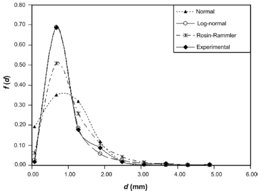
**Figure 2.14:** Comparison between experimental drop size data and selected drop size distribution types in an horizontal pipe flow ( $V_{so} = 0.75\text{m/s}$ ,  $V_{sw}=0.75\text{m/s}$ , oil drops). (Vielma et al., 2008).
