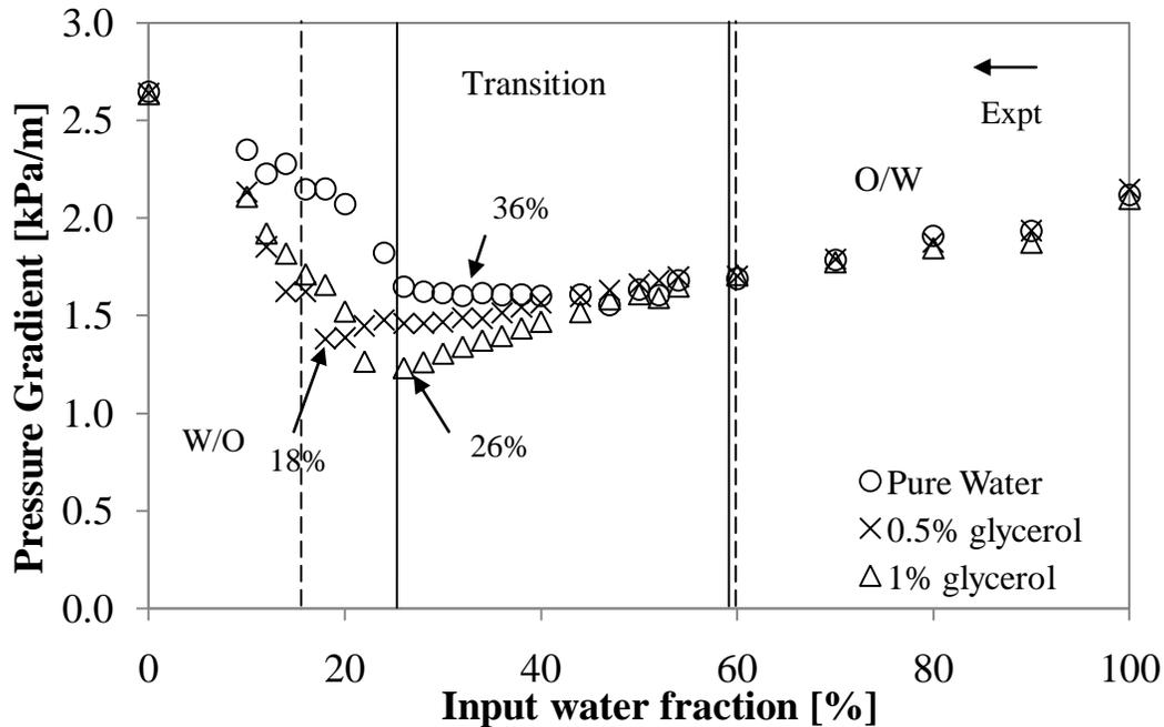
**Figure 5.5:** Experimental pressure gradient for pure water, 0.5% 1% glycerol solutions at different input water fractions at a mixture velocity of 3m/s. The vertical lines indicate the boundaries of the phase inversion transition region for pure water (solid lines) and both glycerol solutions (dotted lines). The percentages indicate the water fractions where pressure gradient shows a minimum. The arrow denotes the direction of experiment from aqueous to oil continuous dispersion.
