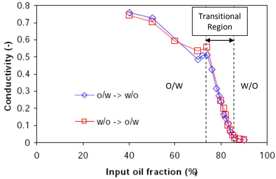
**Figure 2.10:** Conductivity measurement conducted at the centre of a vertical pipe across the phase inversion process (Hu, 2005).
