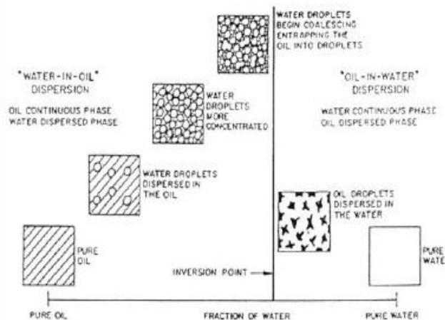
**Figure 2.6:** A schematic on the proposed phase inversion mechanism by Arirachakaran et al. (1989).
