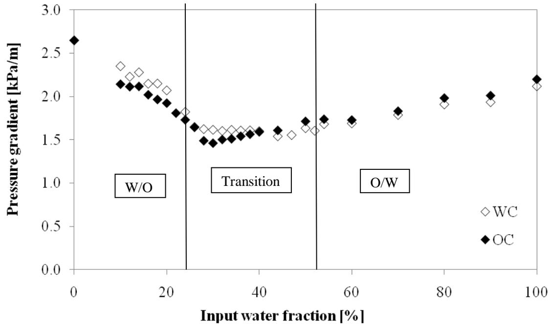
**Figure 4.10:** Comparison of pressure gradient for the oil/water system in an acrylic pipe at a mixture velocity of 3m/s between the two inversion routes (a) starting from oil continuous dispersion (OC) (b) starting from water continuous dispersion (WC). The vertical lines represent the boundaries of the phase inversion transition region.
