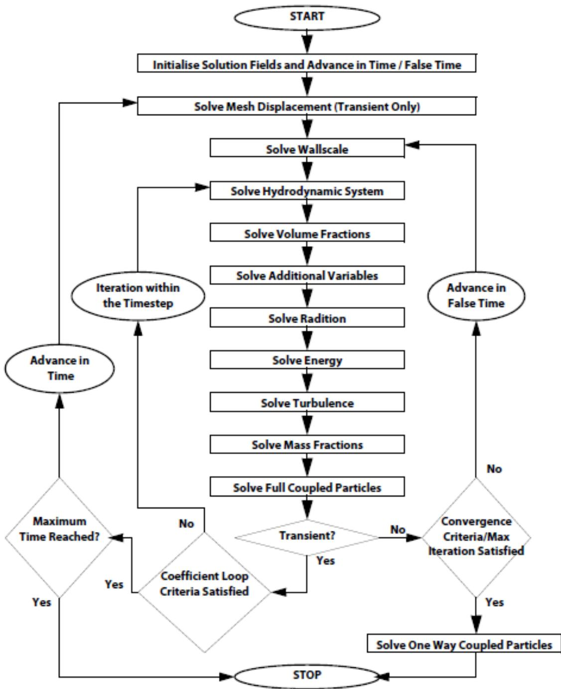
**Figure 8.1:** Schematic diagram on the iterative method for solving the conservation equations (Ansys CFX Manual).
