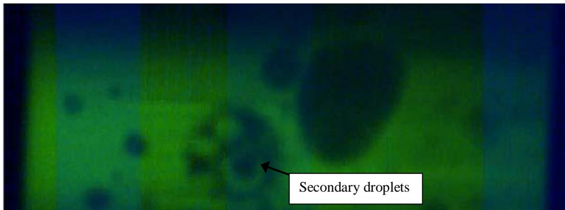
**Figure 2.11:** Multiple dispersions of an oil/water system at a mixture velocity of 1.5m/s and input oil fraction of 31%. The dark region represents the oil phase and the light region represents the water phase. (Liu et al., 2006)
