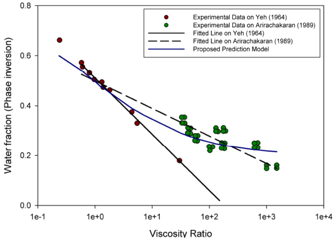
**Figure 6.7:** Application of proposed model on various systems from Yeh et al. (1964) and Arirachakaran et al. (1989). The solid line represents the prediction model by Yeh et al. (1964) (see Equation 6.17) and the dotted line represents the prediction model by Arirachakaran et al. (1989) (see Equation 6.15).
