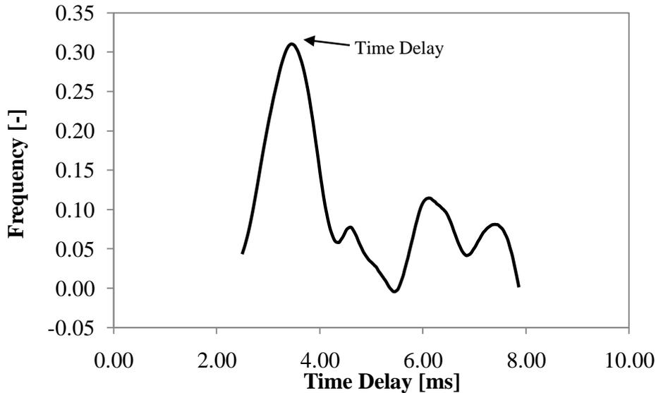
**Figure 3.16:** A sample frequency plot of the time delay between the two impedance wires. The highest peak denotes the time delay where most dispersed drop take to cross the two wires.
