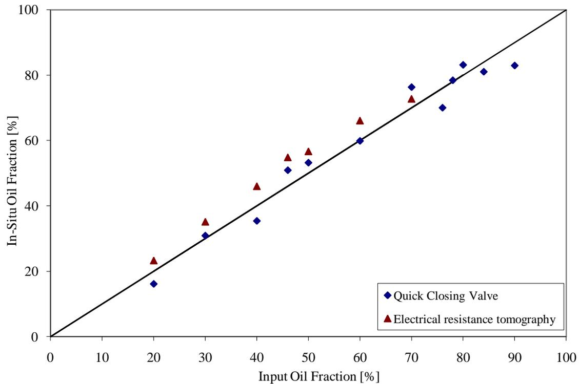
**Figure 3.13:** In-situ liquid hold-up comparison between electrical resistance tomography (ERT) and quick closing valves across a range of input phase fractions at a mixture flow velocity of 3m/s.
