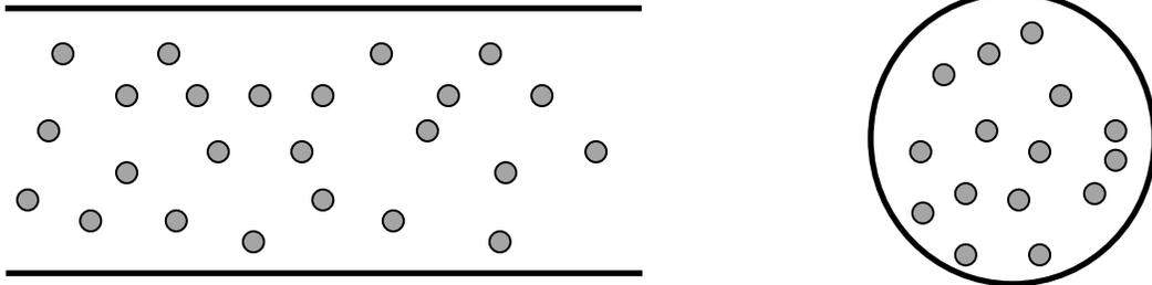
(2) As the oil fraction increases, the oil drops will accumulate at the pipe centre where they coalesce and the mixture inverts.
