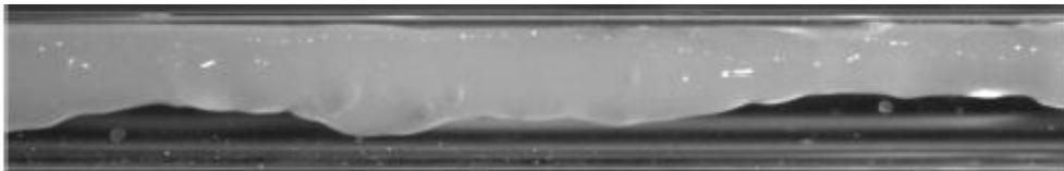
**Figure 2.4:** Annular flow with an oil core and a water annulus. Small amount of drops are also observed within the oil core in the figure. (Ngan et al., 2007)
