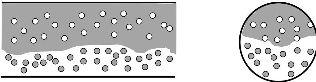
(4) At high oil fractions, the thin layer of water at the bottom of the pipe also disperses and the flow becomes fully dispersed with oil as the continuous phase.
