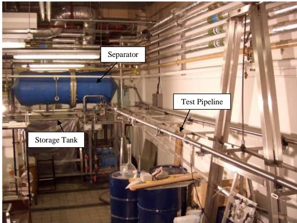
**Figure 3.2:** Photograph of the pilot scale facility in stainless steel.
