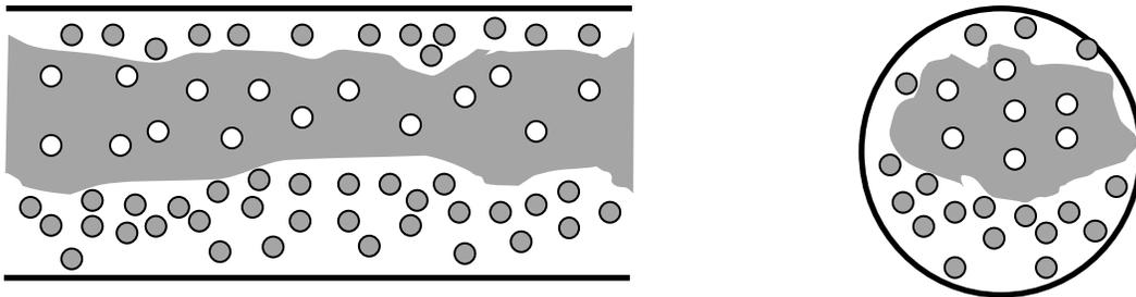
(3) With the mixture also inverts at the top of the pipe, a dual continuous flow pattern is formed with oil as the continuous phase at the top of the pipe and water as the continuous phase at the bottom.
