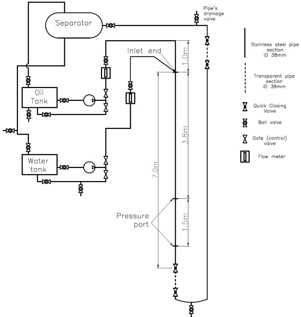
**Figure 3.1:** Schematic of the pilot scale facility with adjustable sections in the test pipeline.
