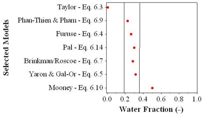
**Figure 6.2:** Predicted inversion points using different dispersion viscosity models against the experimental phase inversion range for a dispersion of water and (a) Exxsol D80 (1.7mPas), (b) Exxsol D140 (5.5mPas), (c) Marcol 52 (11mPas) (data in stainless steel pipe by Ioannou, 2006). Points in graph refer to the model predictions while the lines represent the experimental phase inversion region.
