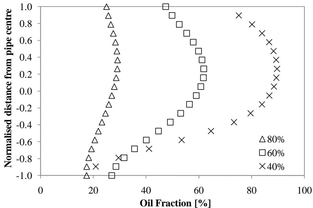
**Figure 8.3:** Experimental oil phase distribution along a vertical pipe diameter at a mixture velocity of 3m/s. Data is extracted from ERT measurements at 7m from the inlet where flow is fully developed.
