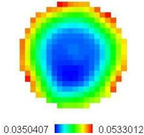
**Figure 3.12:** Sample ERT reconstructed image generated from ITS toolsuite. The colour bar denotes the range of raw conductivity data with respect to the reference frame.
