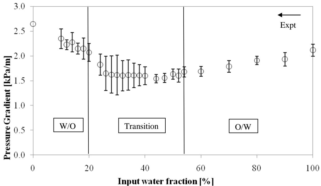
**Figure 4.9:** Experimental pressure gradients in an acrylic pipe at a mixture velocity of 3m/s. The error bars represent the standard deviation of the fluctuations at each specific phase fraction. The arrow denotes the direction of experiment from water continuous to oil continuous dispersion and the vertical lines represent the boundaries of the phase inversion transition region.
