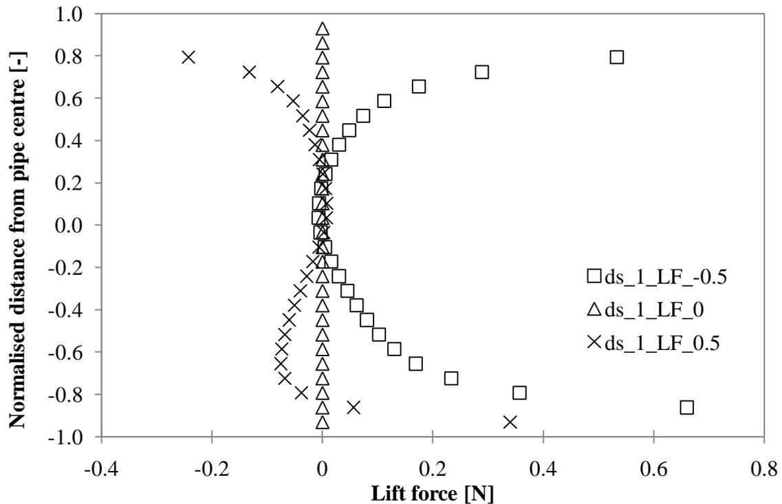
Figure 8.6: Effect of lift force coefficient on the lift force term at a mixture velocity of 3m/s and an input water fraction of 80%. ds represents the drop size in mm and LF represents the lift force coefficient applied to Equation 2.37.
