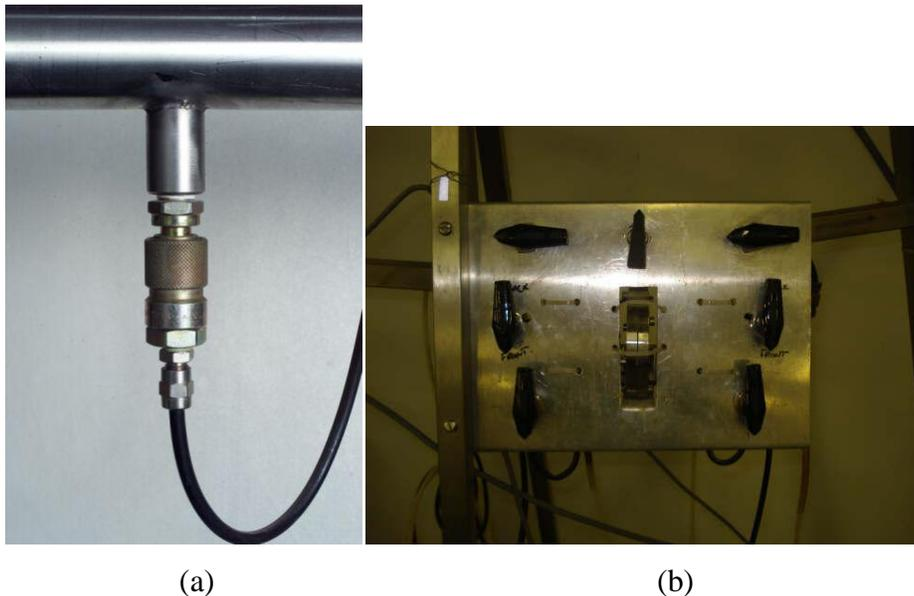
**Figure 3.17:** (a) Pressure measuring port at stainless steel pipeline. Similar ports are also found in the acrylic pipeline (b) Differential pressure transducer and control valves.
