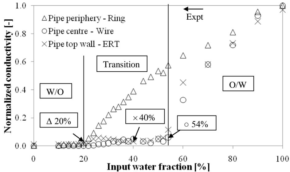
**Figure 4.4:** Normalized conductivity data of the oil/water system in an acrylic pipe at a mixture velocity of 3m/s from the ring and wire probes as well as the ERT system. The vertical lines limit the phase inversion transition region and are drawn at the first and last near zero conductivity values recorded using the various probes. The percentages represent the water fraction at which the different probes show near-zero conductivity values.
