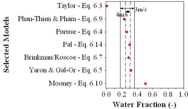
**Figure 6.4:** Predicted inversion points using different dispersion viscosity models against the experimental phase inversion ranges in stainless steel pipe obtained at different mixture velocities for a water-Marcol 52 mixture. Points in graph refer to the model predictions while the lines represent the experimental phase inversion range.
