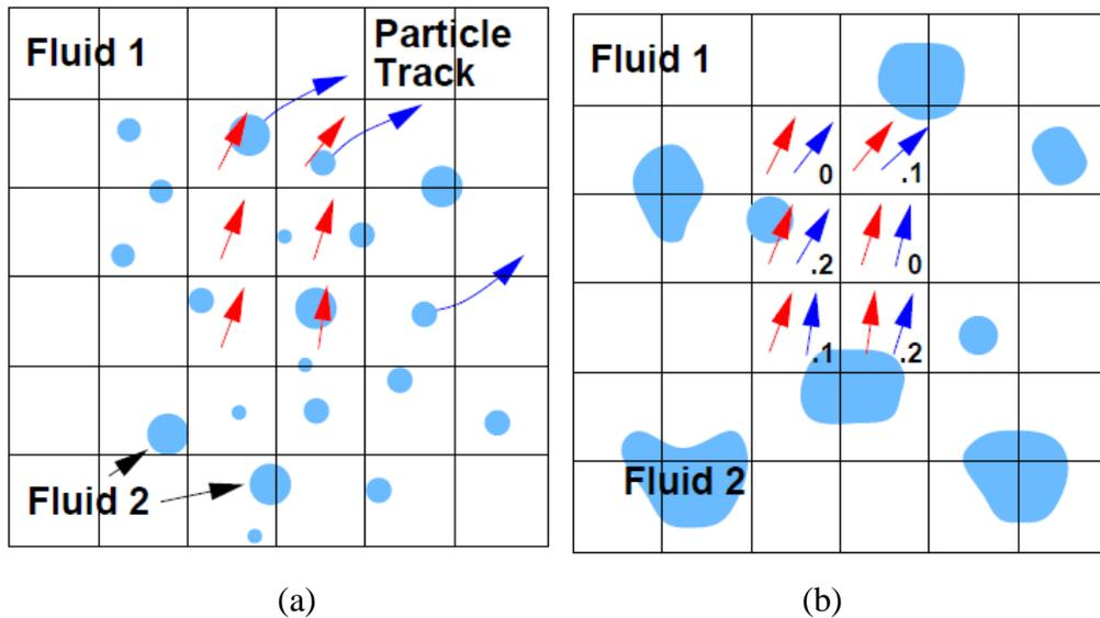
**Figure 2.15:** Schematic representation on the modelling approaches for two-phase flow: (a) Eulerian-Lagrangian approach and (b) Eulerian-Eulerian approach. The number next to the blue arrow in (b) represents the volume fraction of the dispersed phase within the control volume. (Rusche, 2002)
