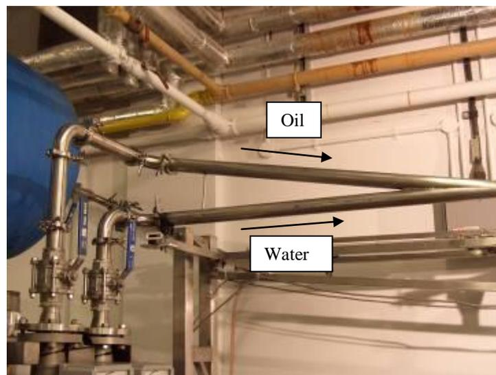
**Figure 3.3:** Stainless steel Y-inlet where the oil and water phases are joined at the end.
