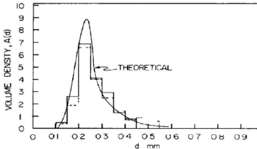
**Figure 2.13:** Comparison between calculated drop size distribution and experimental drop size data. Dotted line represents the histogram at the circulation region and the solid line represents the histogram at the impeller region. (Coulaloglou and Tavlarides, 1977).
