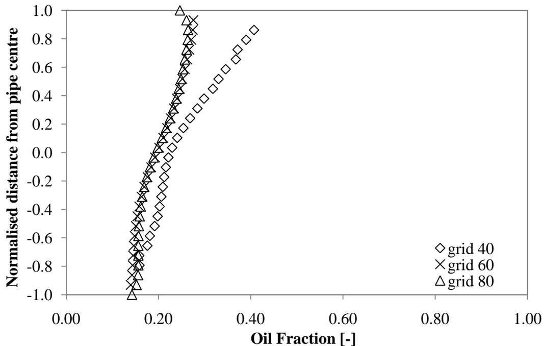
**Figure C-2:** Comparison of results on the dispersed phase fraction along a vertical diameter at the end of the pipe with 3m in length. An input dispersed phase fraction of 0.2 is chosen for all 3 cases.
