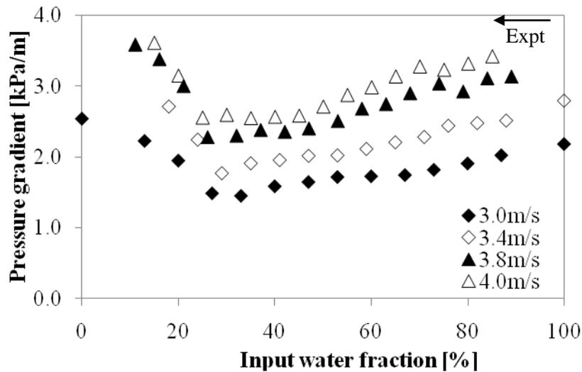
**Figure 4.12:** Comparison of pressure gradient measurement between mixture velocity of 3m/s and 4m/s in a stainless pipe. The arrow denotes the direction of experiment from water continuous dispersion to oil continuous dispersion.
