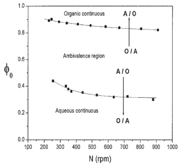
**Figure 2.7:** The existence of ambivalent region between the aqueous and organic continuous dispersion across the organic phase fraction ( $\Phi_o$ ) (Noui-Mehidi et al., 2004).
