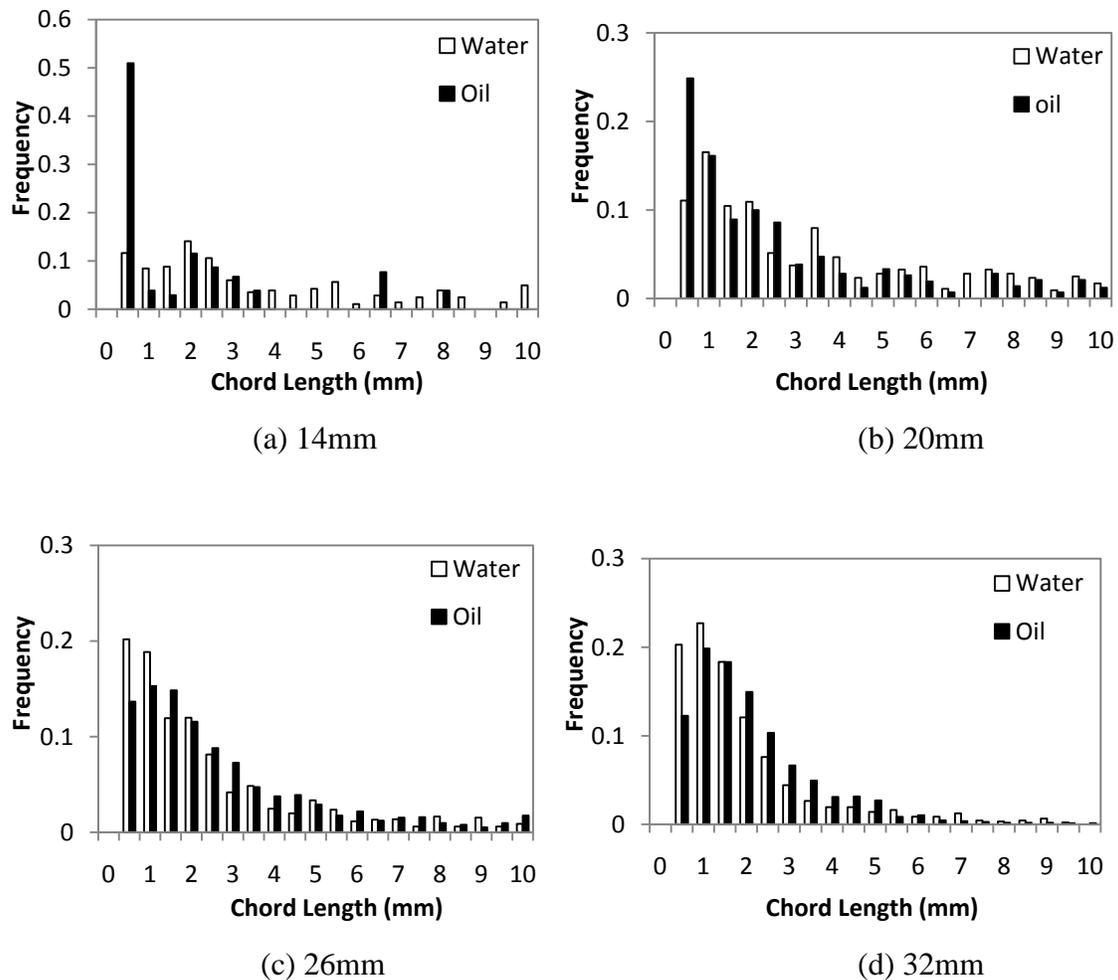
**Figure A-1:** Chord length distribution of oil drops in water (54% water fraction) at various locations from the top wall of the pipe with a mixture velocity of 3m/s. The distributions of the two inversion routes are given – starting from a O/W dispersion (□) and from a W/O dispersion (■).
