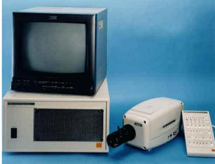
**Figure 3.7:** Setup of the high speed video imaging unit, Kodak HS 4540 MX.
