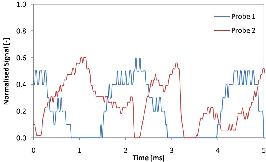
**Figure 3.15:** A sample set of normalized signal from the two impedance wires at a mixture velocity of  $3\text{m/s}$ . Dispersed phase will be in contact with probe 1 before it contacts with probe 2.
