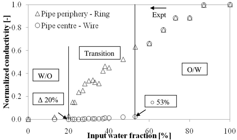
**Figure 4.5:** Normalized conductivity data of the oil/water system in a stainless steel pipe at a mixture velocity of 3m/s from the ring and wire probes as well as the ERT system. The vertical lines limit the phase inversion transition region and are drawn at the first and last near zero conductivity values recorded using the various probes. The percentages represent the water fraction at which the different probes show near-zero conductivity values.
