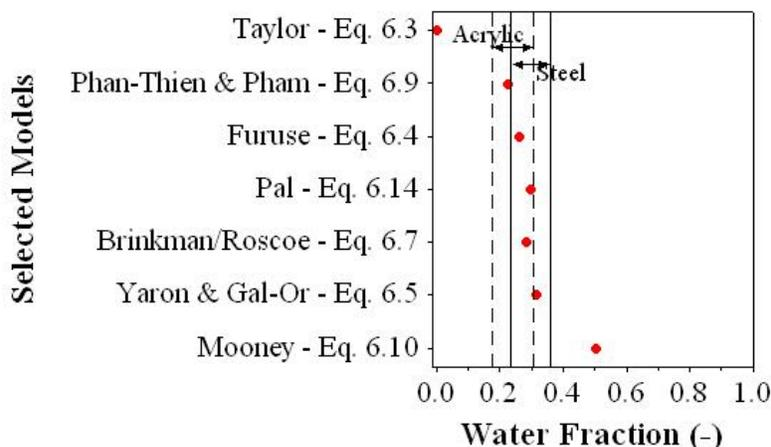
**Figure 6.5:** Predicted inversion points using different dispersion viscosity models against the experimental phase inversion ranges obtained with different test sections for a water-Marcol 52 mixture. Points in graph refer to the model predictions while the lines represent the experimental phase inversion range.
