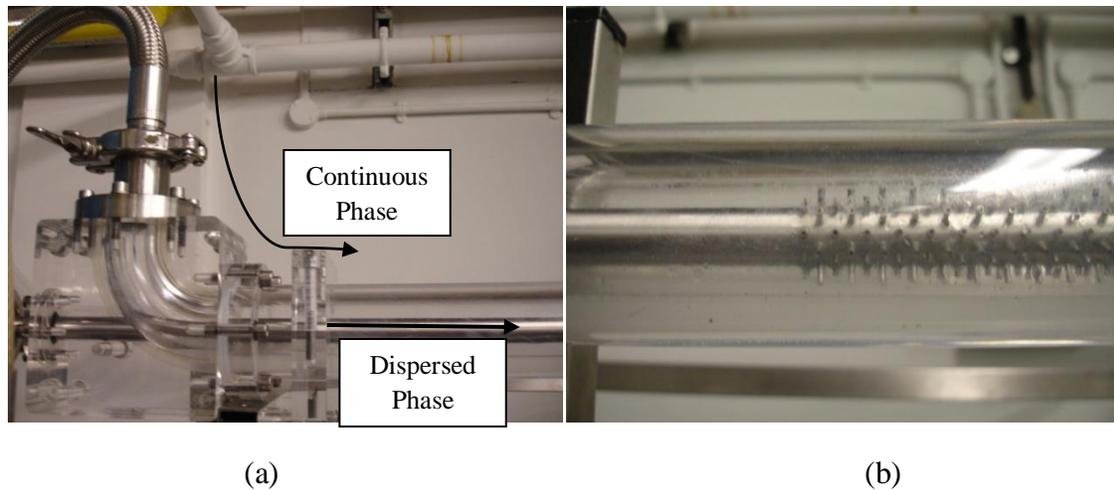
**Figure 3.5:** Dispersion inlets with staggered nozzles. (a) The dispersed phase flows within the stainless steel pipe while the continuous phase flows in the acrylic pipe. (b) Dispersed phase is ejected from the nozzles.
