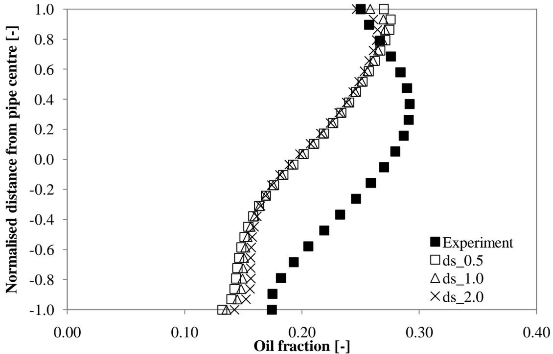
**Figure 8.7:** Effect of drop size on phase distribution at a constant lift coefficient ( $LF=0.5$ ) at a mixture velocity of  $3\text{m/s}$  and input water fraction of  $80\%$ .  $ds$  represents the drop size in  $\text{mm}$ .
