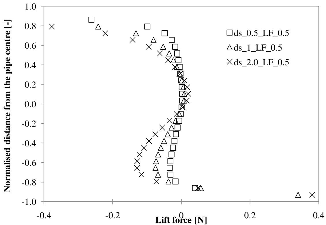
**Figure 8.8:** Effect of drop size on the lift force of a constant lift coefficient (LF=0.5) at a mixture velocity of 3m/s and input water fraction of 80%. ds represents the drop size in mm.
