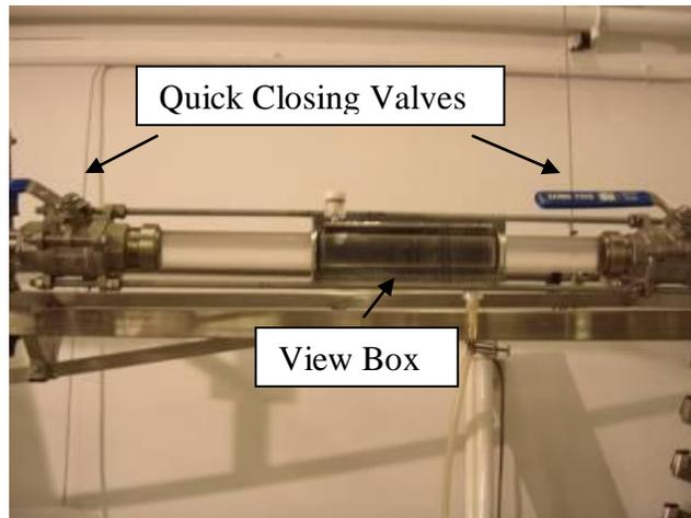
**Figure 3.8:** Section of pipe with quick closing valves in the 38mm stainless steel pipeline. A viewbox is included to aid visual observation and video capturing.
