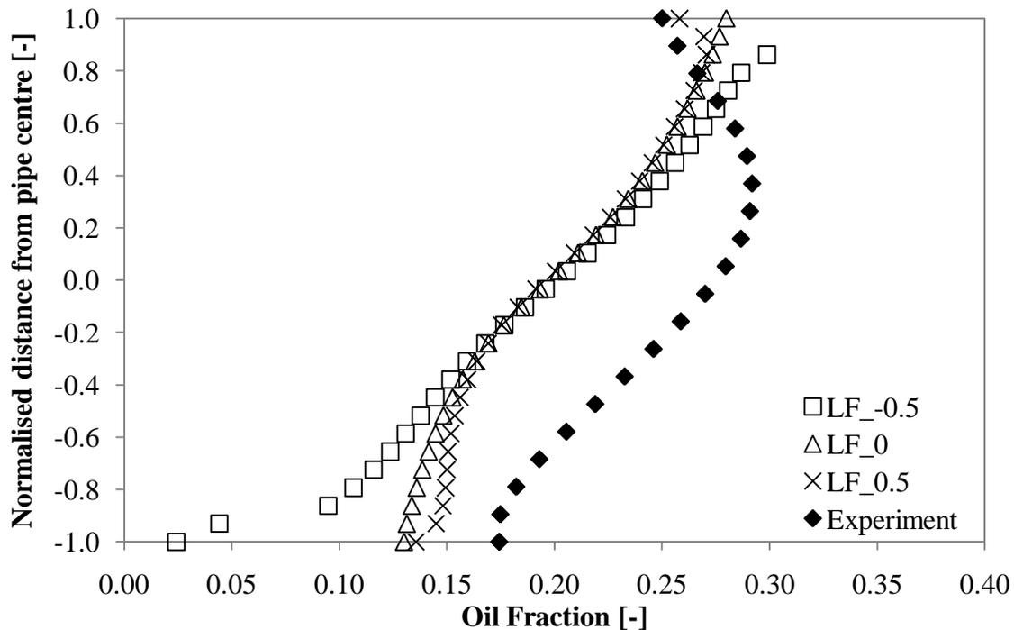
**Figure 8.5:** Effect of lift force on phase distribution at mixture velocity of 3m/s and input water fraction of 80%. LF in the legend represents the lift coefficient applied to Equation 2.37.
