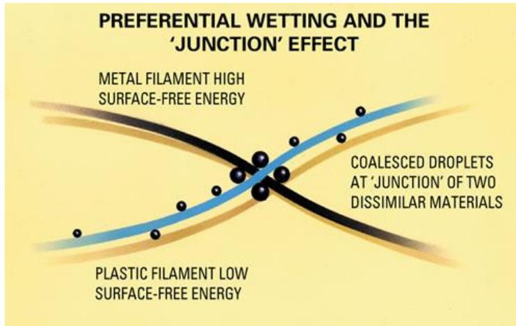
**Figure 3.6:** Junction effect of the coalescer that enhances separation. (Information from manufacturer - KnitMesh Technologies).
