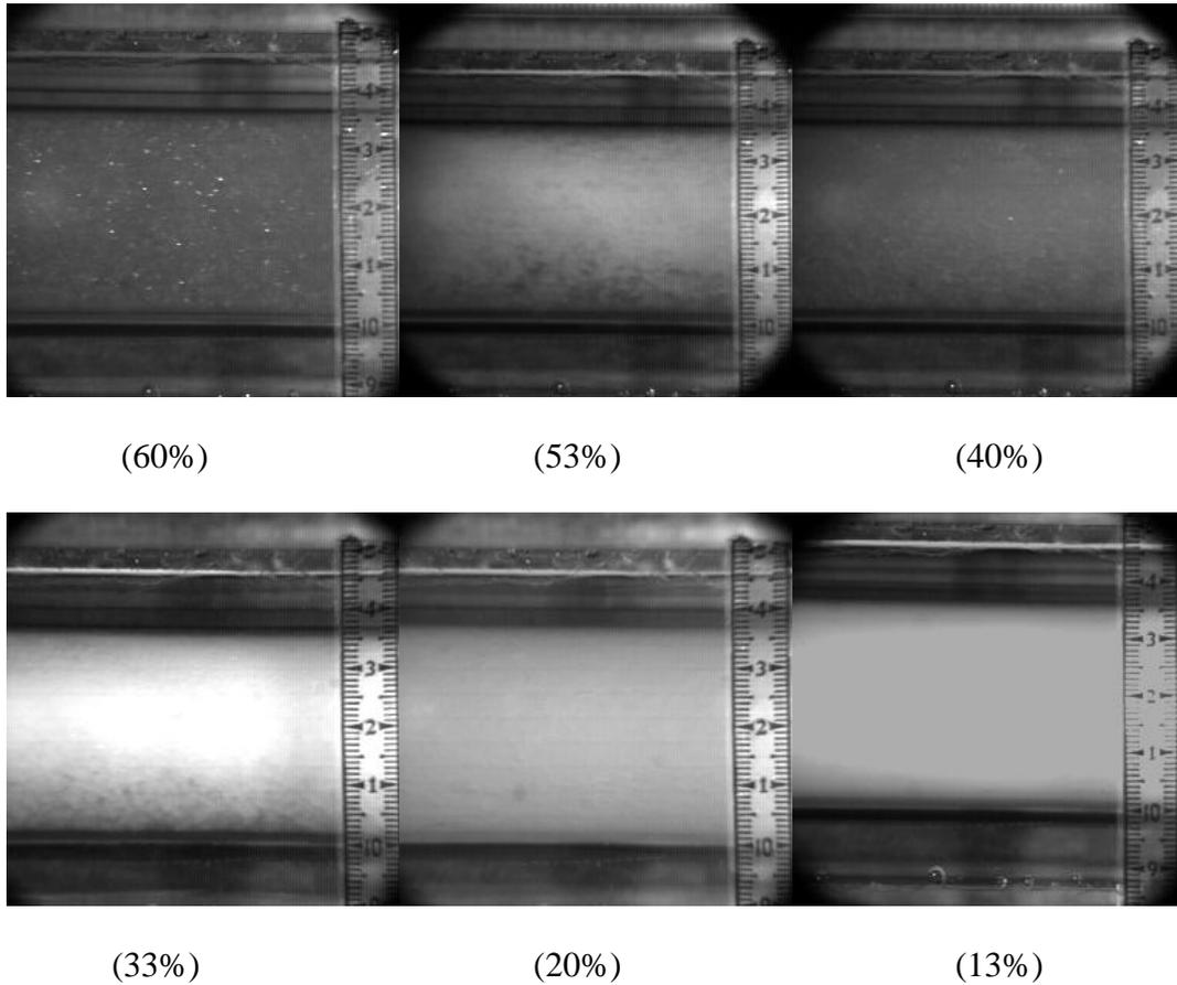
**Figure 4.1:** Visual images are taken in a stainless steel pipe using an high speed camera (Model: Vision Research Phantom V5.1) at 7m away from the inlet. Mixture velocity is kept constant at 3m/s. The percentage in the bracket represents the input water fraction which the image is taken.
