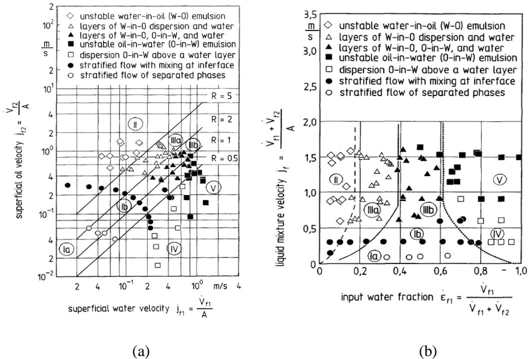
**Figure 2.1:** (a) Flow regime map that is based on the fluid superficial velocities (b) Flow regime map that is based on input water fraction and mixture velocity.
