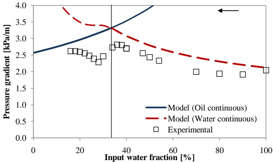
**Figure 6.8:** Comparison of pressure gradient at different phase fraction between experimental data ( $\square$ ) and modeling outcome via Brinkman/Roscoe (1952)'s mixture viscosity correlation. The solid arrow ( $\leftarrow$ ) represents the direction for the experiment and the vertical line denotes the predicted phase inversion point.
