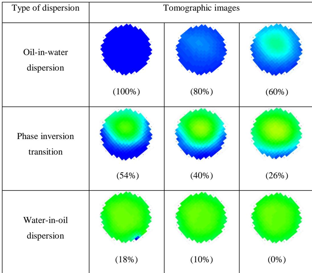
**Figure 4.3:** Phase distribution in an acrylic pipe cross section during the transition from a water continuous to an oil continuous mixture at a mixture velocity of 3m/s. The percentages in brackets represent the input water fraction.
