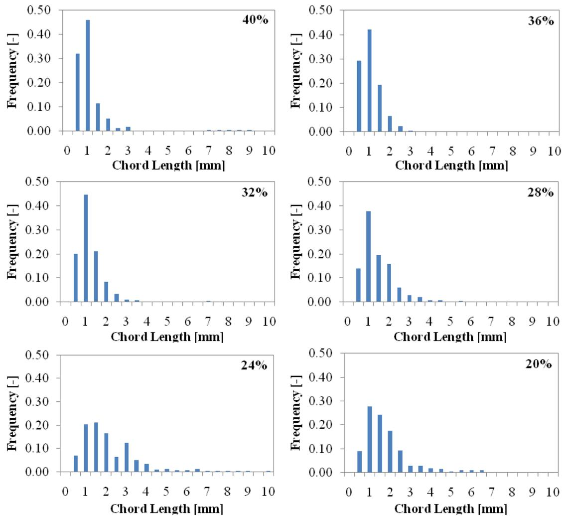
Figure 4.19 Comparison of chord length distribution at different input water fraction (fraction in bracket) across the phase inversion process at 3m/s mixture velocity.
