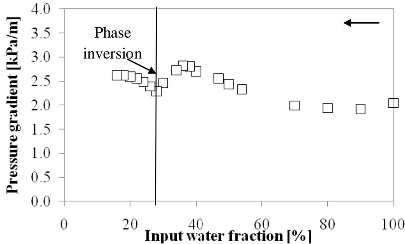
**Figure 4.18:** Experimental pressure gradients for a dispersed inlet configuration at a mixture velocity of 3m/s. The arrow denotes the direction of experiment from water continuous to oil continuous dispersion and the vertical line represents the phase inversion point.
