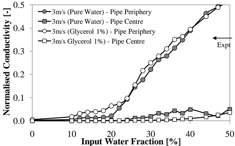
**Figure 5.3:** A comparison of the normalised conductivities in the middle of the pipe and the pipe periphery between the 1% glycerol solution and the pure water dispersions at a mixture velocity of 3m/s.
