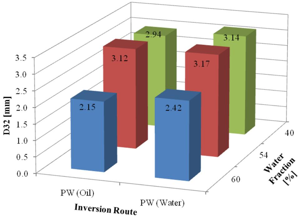
**Figure 4.15:** Sauter mean diameter at different input water fraction across the phase inversion boundary (1). The phase in brackets represents the initial continuous phase and the number in each column represents the Sauter mean diameter at the specific sample.
