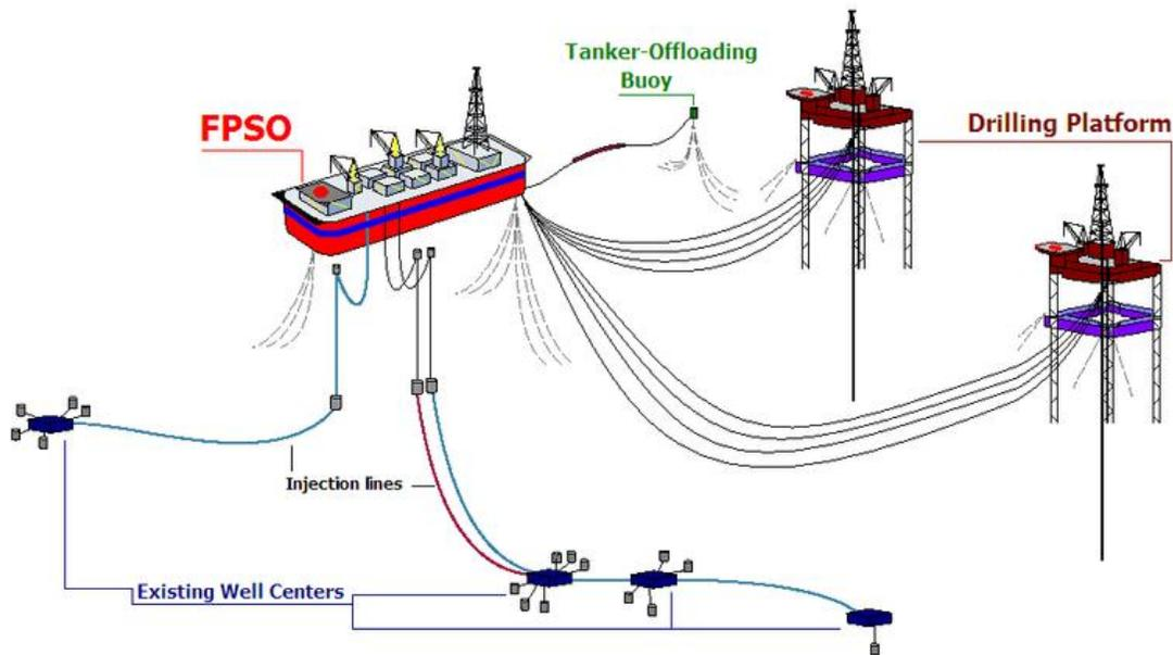
Figure 1.1 Offshore production pipeline schematic from well centres to production platforms and FPSO.
