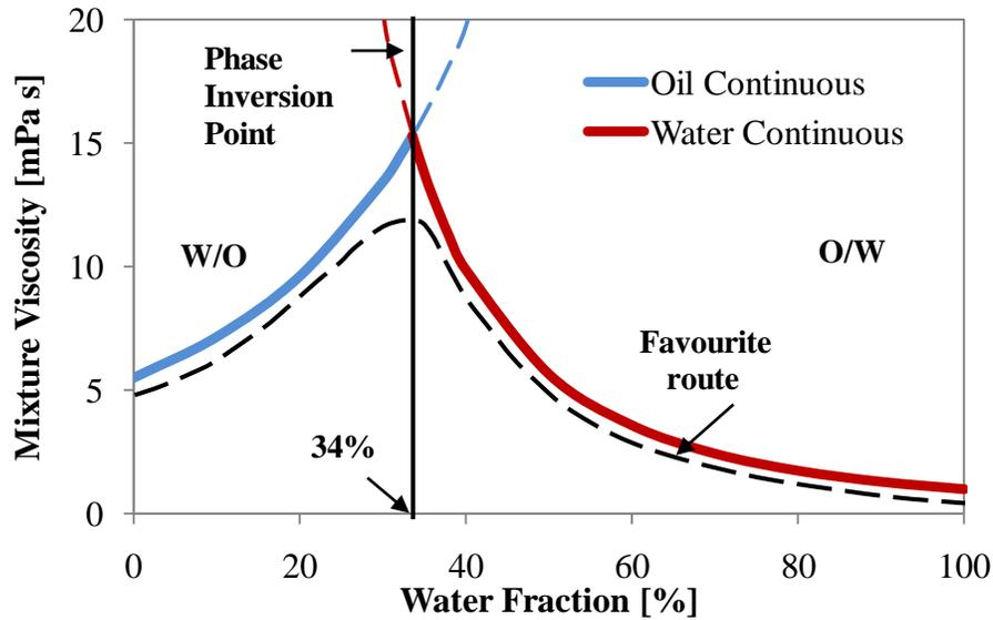
**Figure 6.1:** Prediction of phase inversion point for the Exxsol D140-water dispersion. Phase inversion occurs at the phase fraction where the difference in viscosity between the oil continuous and the water continuous dispersions becomes 0. The Brinkman/Roscoe (1952) model is used for calculating the viscosity of the dispersions.
