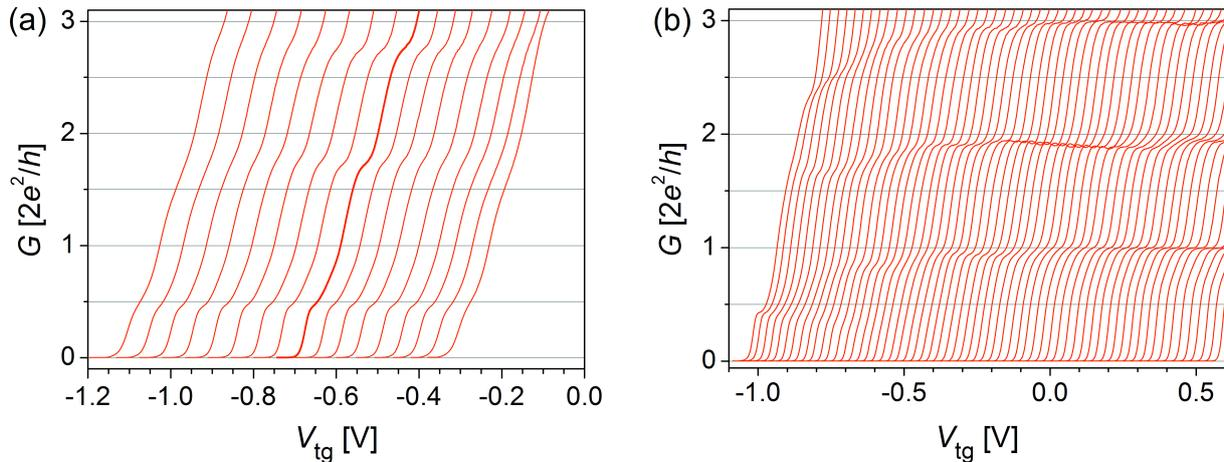
**Figure 3.** (a) Behaviour of the  $e^2/h$  plateau when the channel is shifted laterally by differentially biasing the split gates. (Successive traces have been offset from the central bold trace, which corresponds to equal bias on the two split gates.) The left- and rightmost traces correspond to a differential bias of  $\Delta V_{\text{sg}} = \pm 320$  mV. (b) Conductance traces of the same device after it has been briefly illuminated with an infrared LED to raise the carrier density.
