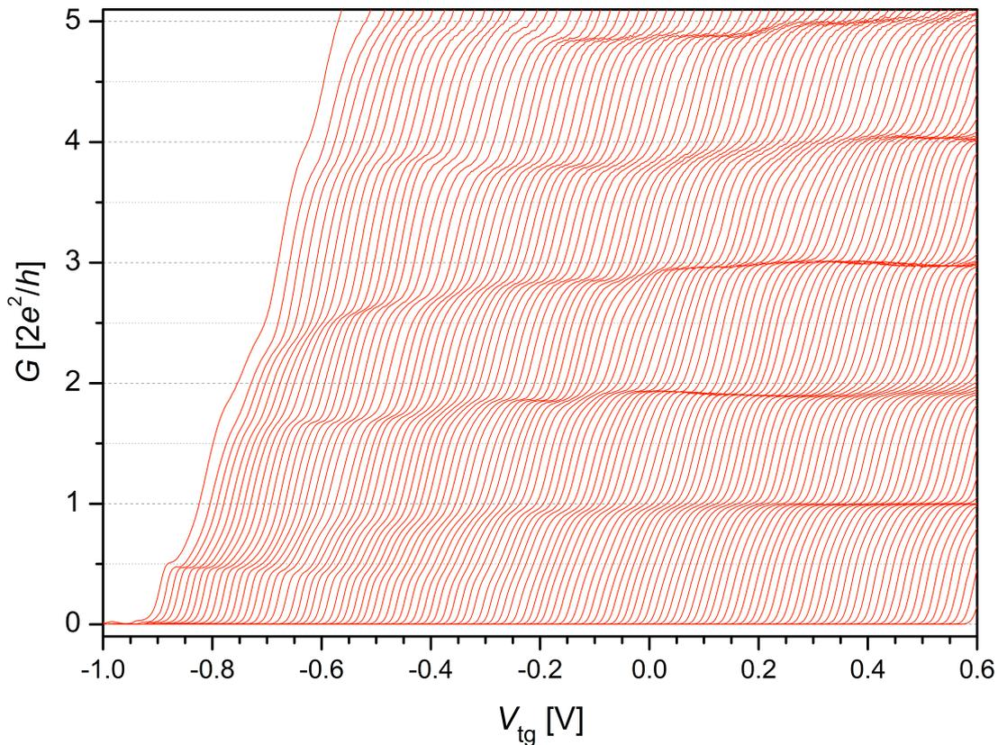
**Figure 1.** Differential conductance traces  $G(V_{tg})$  measured by sweeping  $V_{tg}$  at various fixed  $V_{sg}$ . Moving left-to-right, each successive trace corresponds to a slightly more negative  $V_{sg}$ , i.e., increasing 1D confinement. The régime of strong confinement is therefore to be found on the right, and that of weak confinement on the left.
