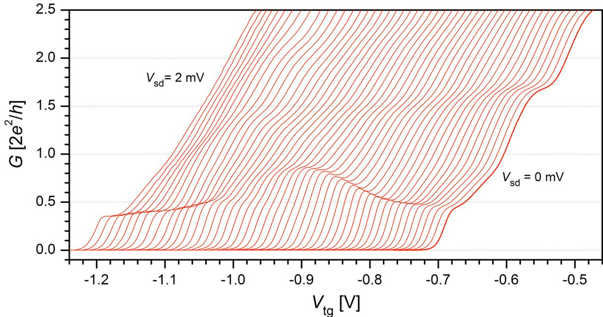
**Figure 2.** Differential conductance traces  $G(V_{tg})$  in the régime of weak confinement showing the evolution of the  $e^2/h$  plateau when a d.c. bias is applied between the source and drain ohmic contacts. The rightmost (bold) trace was taken with no bias applied, with increasing bias up to  $V_{sd} = 2\text{mV}$  on the far left. (Successive traces have been offset from the  $V_{sd} = 0\text{ mV}$  trace for clarity.)
