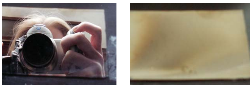
Figure 4.16 Digital photographs illustrating the high reflectivity (left) and gold appearance on the leading edge (right) of TiAs films deposited via the APCVD of [\text{Ti}(\text{NMe}_2)_4] and {}^t\text{BuAsH}_2 .
