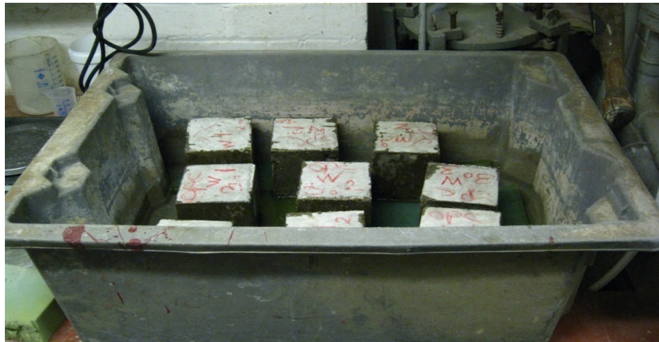
Figure 3.2: Concrete specimens located on synthetic foam in a tray containing salt solution
