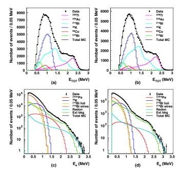
FIG. 1 (color online). Energy sum distribution for crossing-electron events for (a)  $^{130}\mathrm{Te}$  and (b)  $^{\mathrm{nat}}\mathrm{Te}$  (b); Energy distribution of electron events coming from the source foil for (c)  $^{130}\mathrm{Te}$  and (d)  $^{\mathrm{nat}}\mathrm{Te}$ . Dots correspond to the data and histograms to the fit of the background model.
