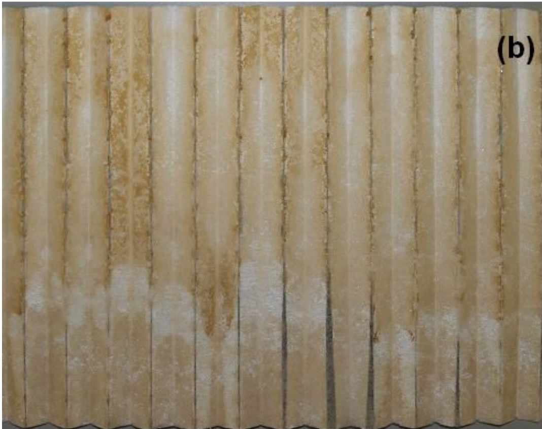
Figure 4-8: Photographs of fouled membrane surfaces from 10" EAV 10,1 cartridge containing tightly packed pleats. The images are taken from two separate cartridges, where (a) is the same image shown in Figure 4-5(b). Membranes imaged as described in Section 2.5.
