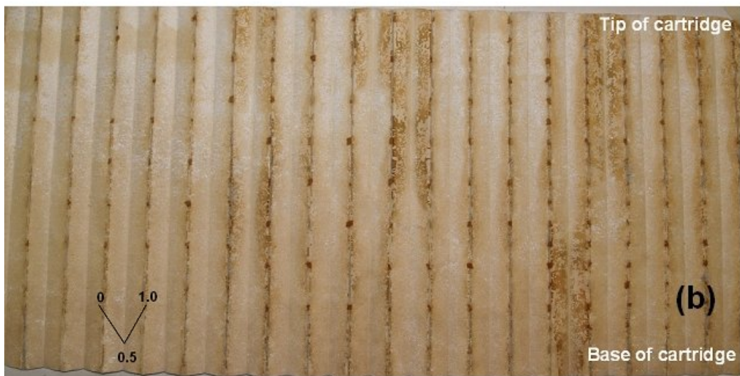
Figure 4-5: Typical photographs of fouled membrane surfaces from 10" module configurations of varying h_p showing yeast cell deposition. Inset shows the position within the pleat, where 0 and 1 indicate the apex of the pleat, 0.5 indicates the base of the pleat. (a) 10" UEAV 24,1 cartridge containing tightly packed pleats of h_p = 24 mm; areas of clean membrane are clearly visible corresponding to the inner surfaces of each pleat. (b) 10" EAV 10,1 cartridge containing Fan pleats of h_p = 10 mm; similar areas of clean membrane are also seen on the inner surface of each pleat. Membranes imaged as described in Section 2.5.
