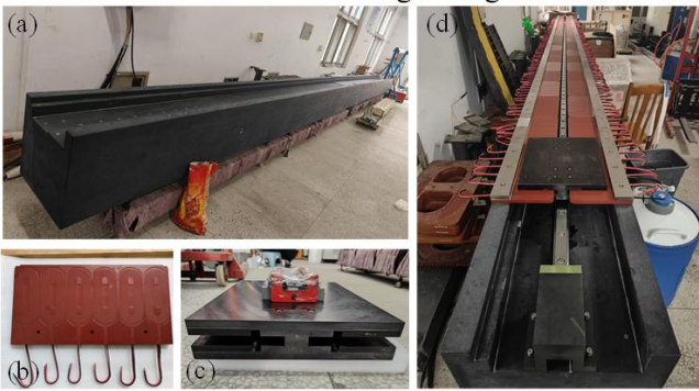
Fig. 24. Full-scale UAV electromagnetic launch platform. (a) Granite foundation. (b) Coil module. (c) Halbach PM array move. (d) PMLB prototype.
