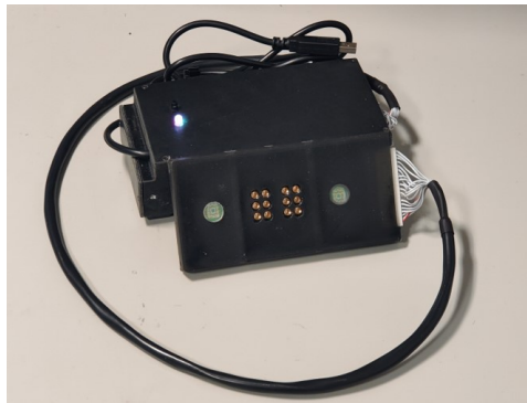
Fig. 1. Image of the FetalSenseM device, with sensor module displaying LED groups and detectors.
