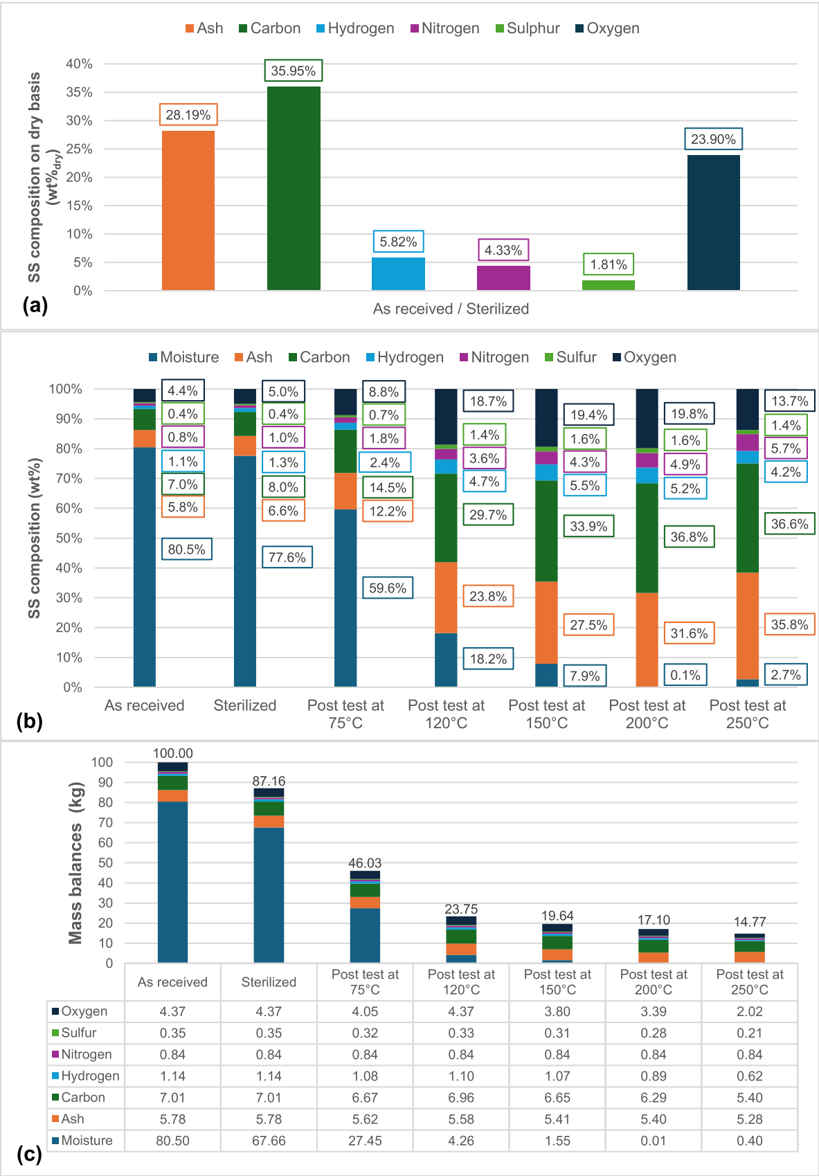
Fig. 1. Composition of SS ar and SS st on dry basis (a); Compositions of SS in different states (b); Mass balances with 100 kg of as-received SS as the reference (c).
