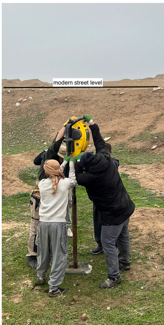
Fig. 3. Coring at the Ishtar Temple in Assur using the Cobra Pro TT corer for sediment column recovery. The modern street level is indicated.
